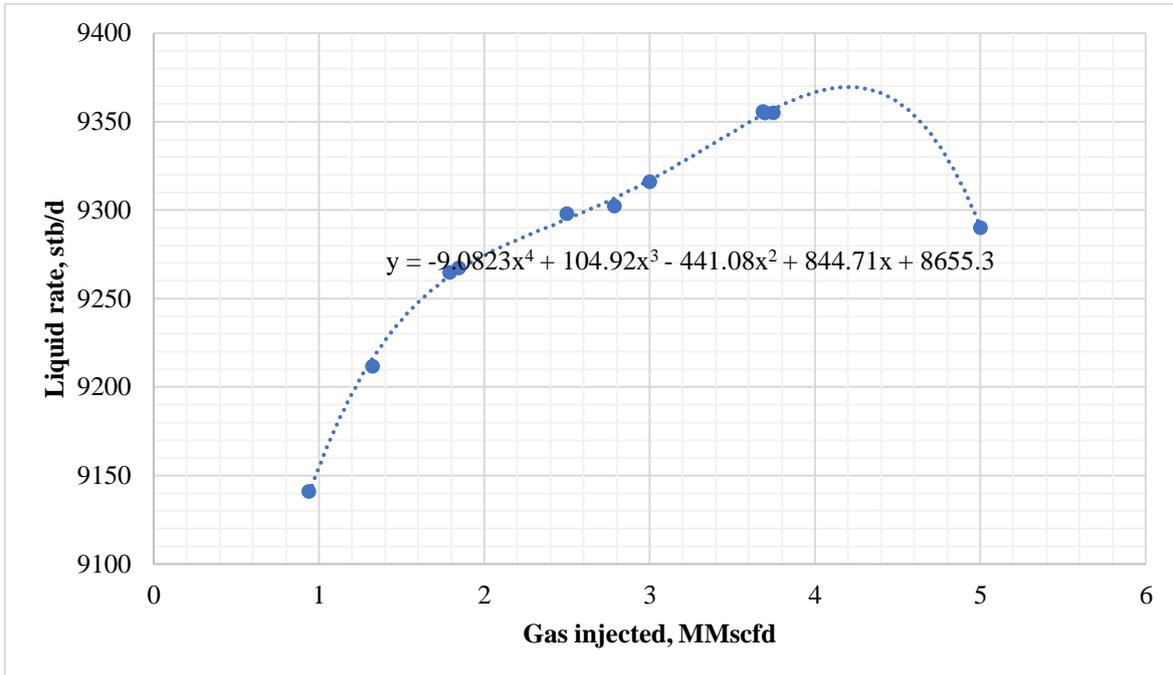
Fig. 7: Liquid Rate Vs Liftgas Injection Rate for Well 1
