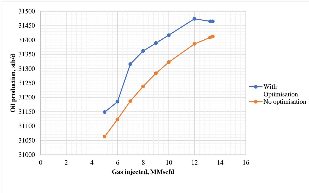
Fig. 11: Comparison Of Field Network Solved With And Without Optimization In Gap
