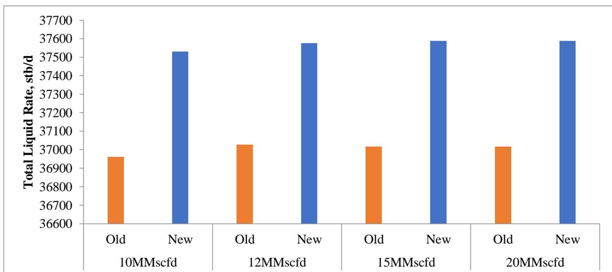
Fig. 18: Comparison Of Total Liquid Rate for Old and New Architectures for The Gaslift Field Production System Network
