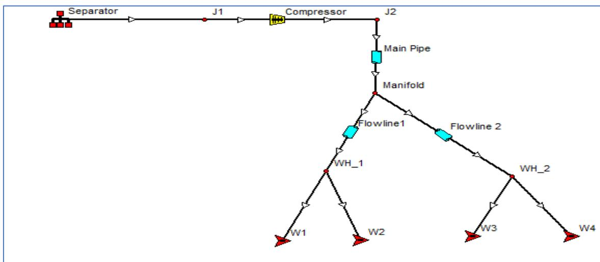
Fig. 3: The Gaslift System Injection Network in Gap
