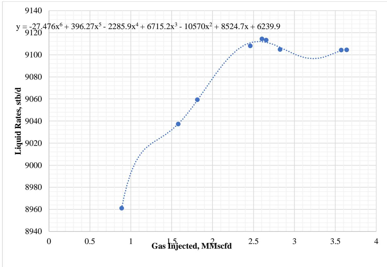
Figure 9: Liquid Rate Vs Liftgas Injection Rate for Well 3
