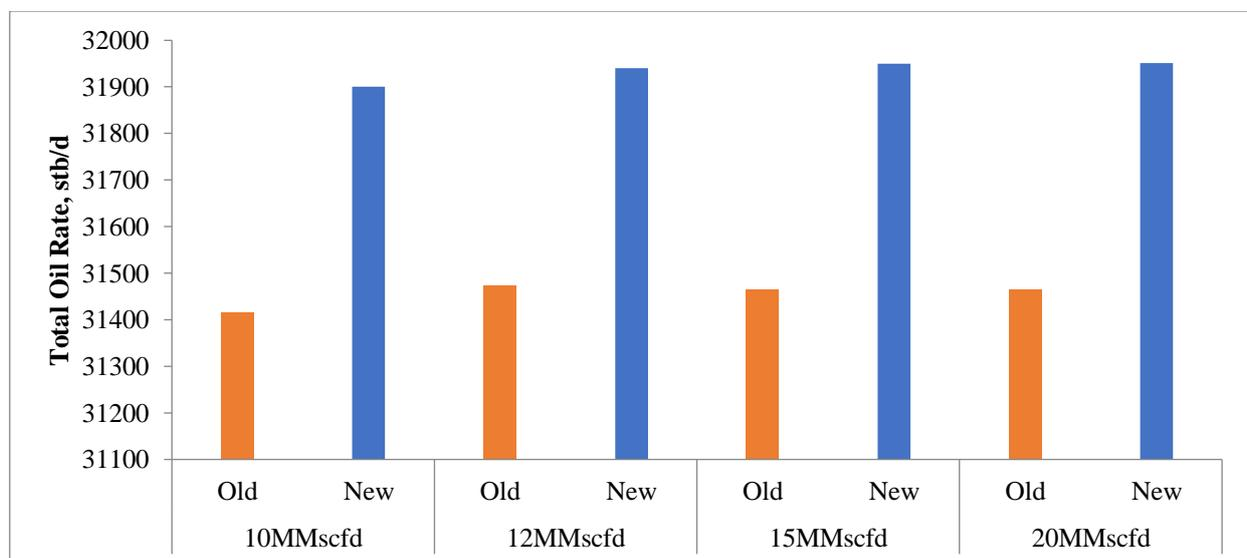
Fig. 16: Comparison Of Total Oil Rate of Old and New Architectures For The Gaslift Field Production System Network
