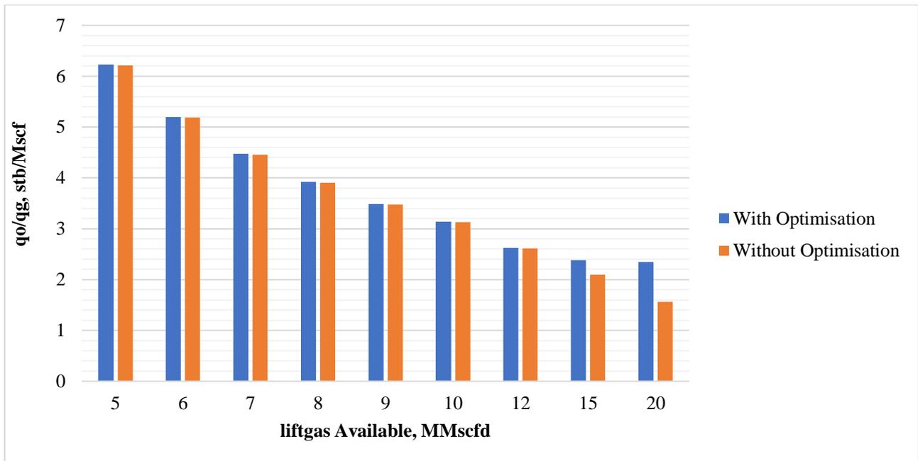
Fig. 15: Chart Showing Oil Produce and Injected Gas Ratio for Various Liftgas Availability
