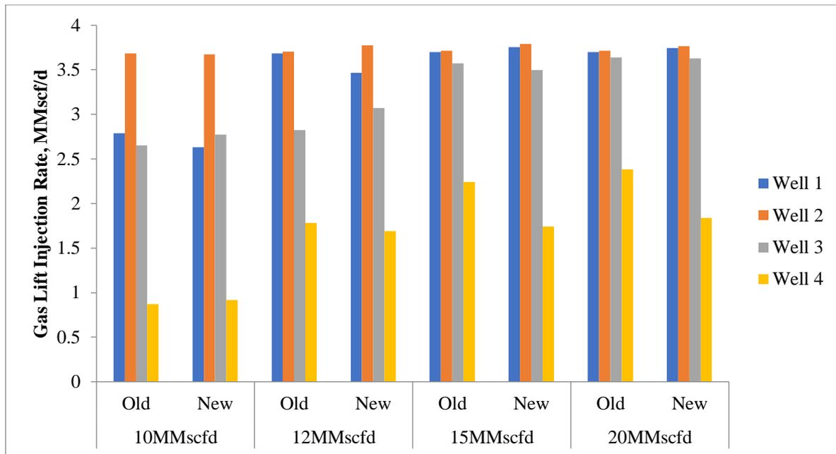
Fig. 21: Comparison Of Liftgas Injection Rate of Individual Wells for The Old and New
