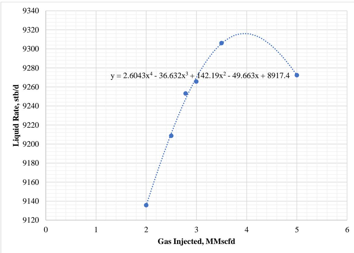
Fig. 8: Liquid Rate Vs Liftgas Injection Rate for Well 2
