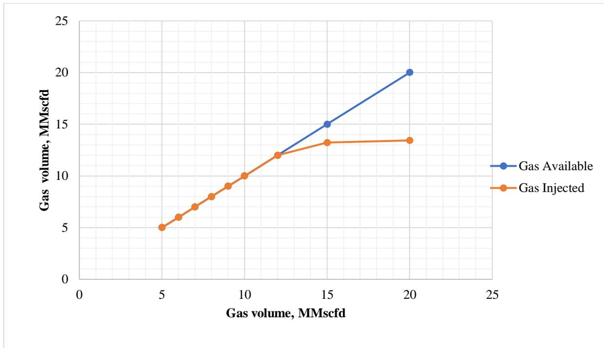
Fig. 13: Comparison Of Gas Available and Gas Utilized for Injection in The Network System Optimization in Gap.
