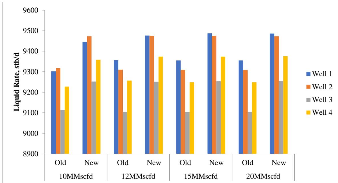
Fig. 19: Comparison Of Individual Well Liquid Rates Between Old and New Network Architectures
