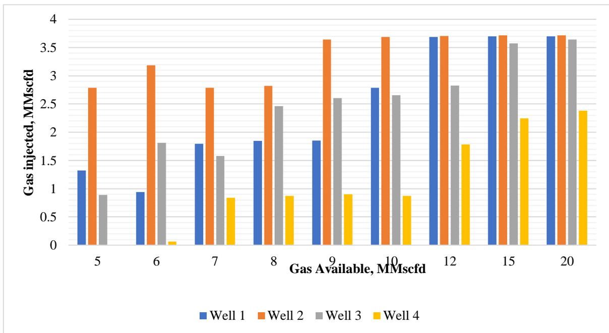
Fig. 14: Gas Injected Vs. Liftgas Available (With Optimization)
