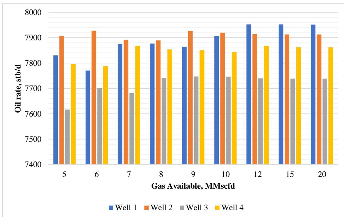
Fig. 12: Oil Rate Vs Liftgas Available (With Optimization)
