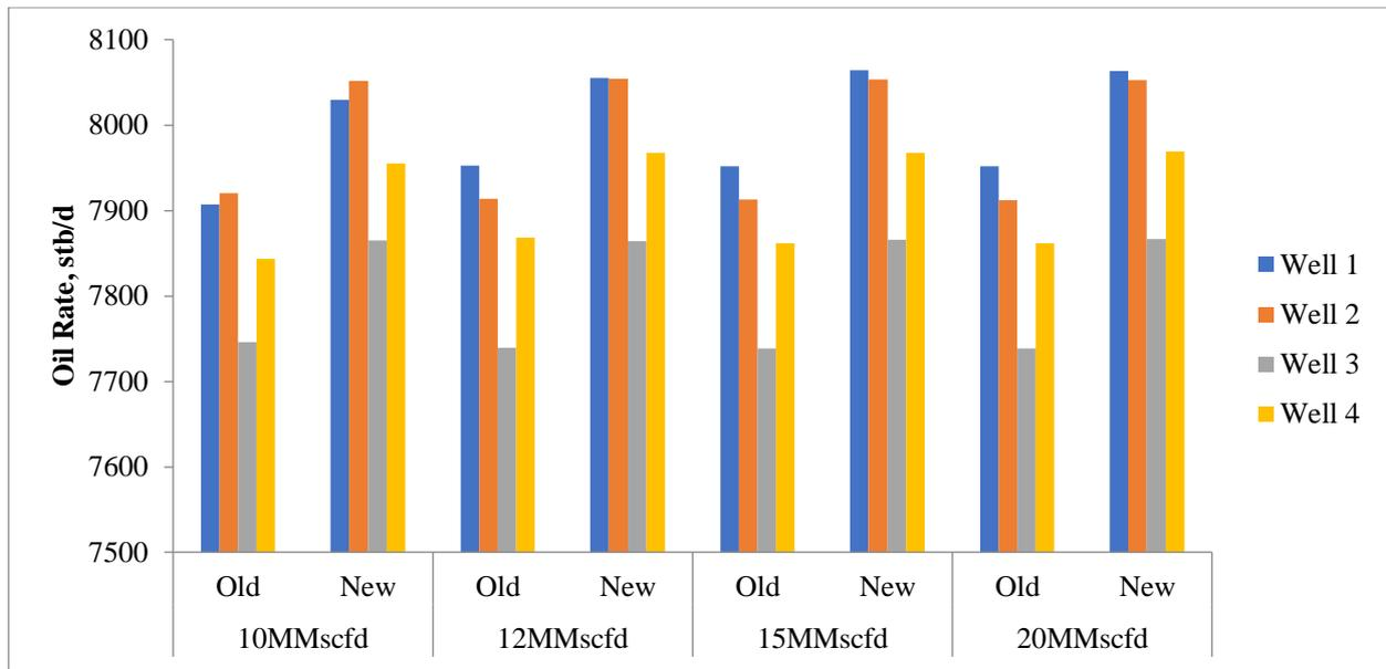
Fig. 17: Comparison of Individual Well Oil Rates Between Old and New Network Architectures
