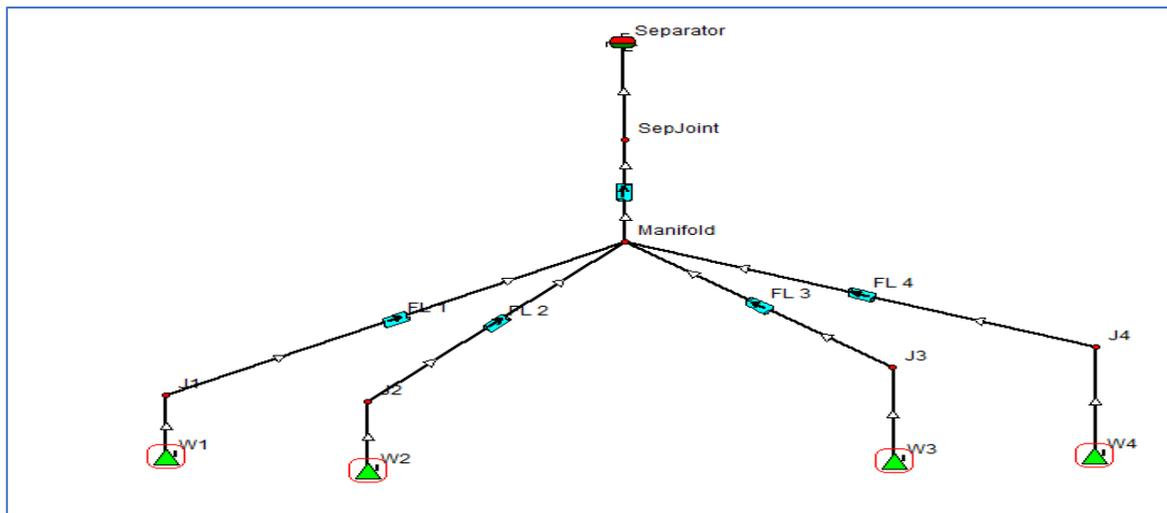
Fig. 4: Redesigned (New) Gaslift Field Production System Network
