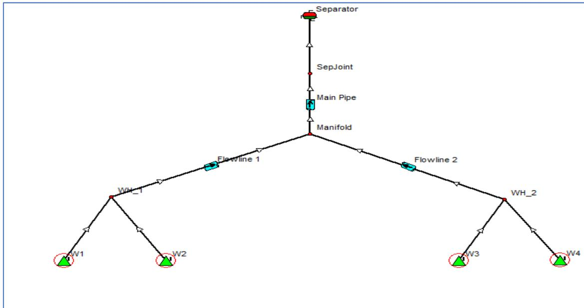
Fig. 2: The Gaslift System Production Network in Gap
