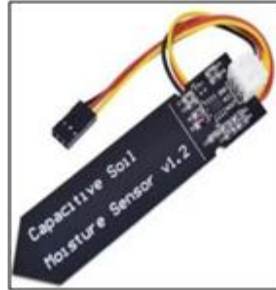
Fig 9 Capacitive Moisture Sensor
