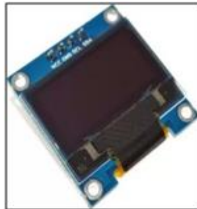
Fig 10 0.96 inch OLED Display
