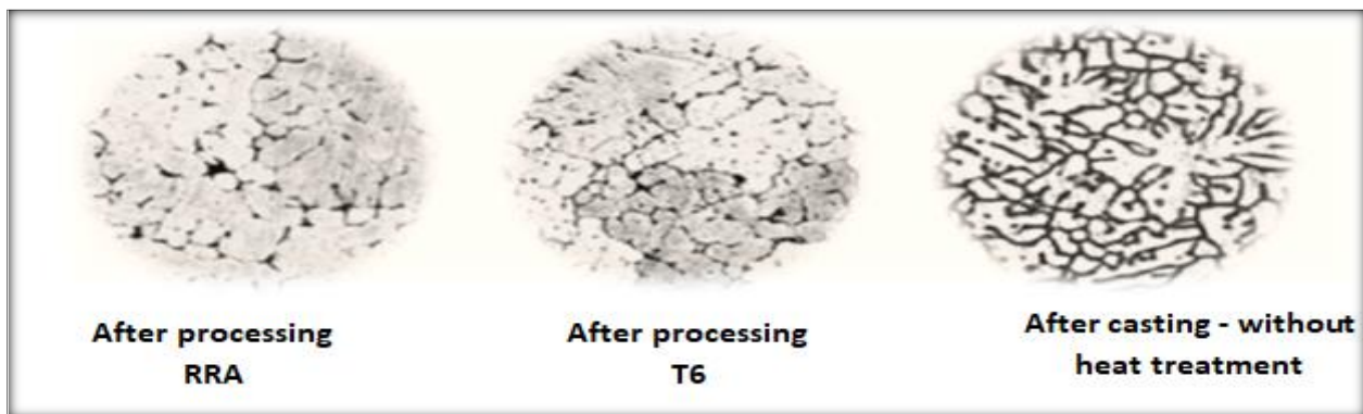
Fig 7 Micrographs at X200 Magnification of Alloy 7075 with 0.1% Nickel Added after Applying Various Heat Treatments
