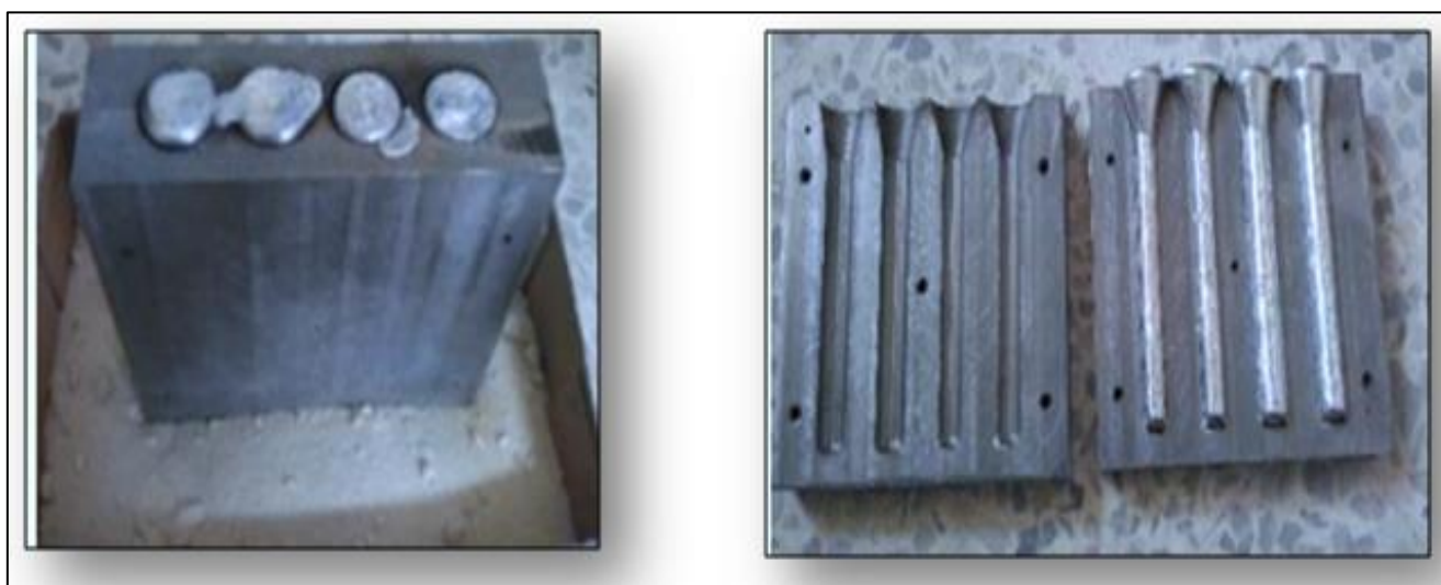
Fig 1 The Steel Mold used for Casting
