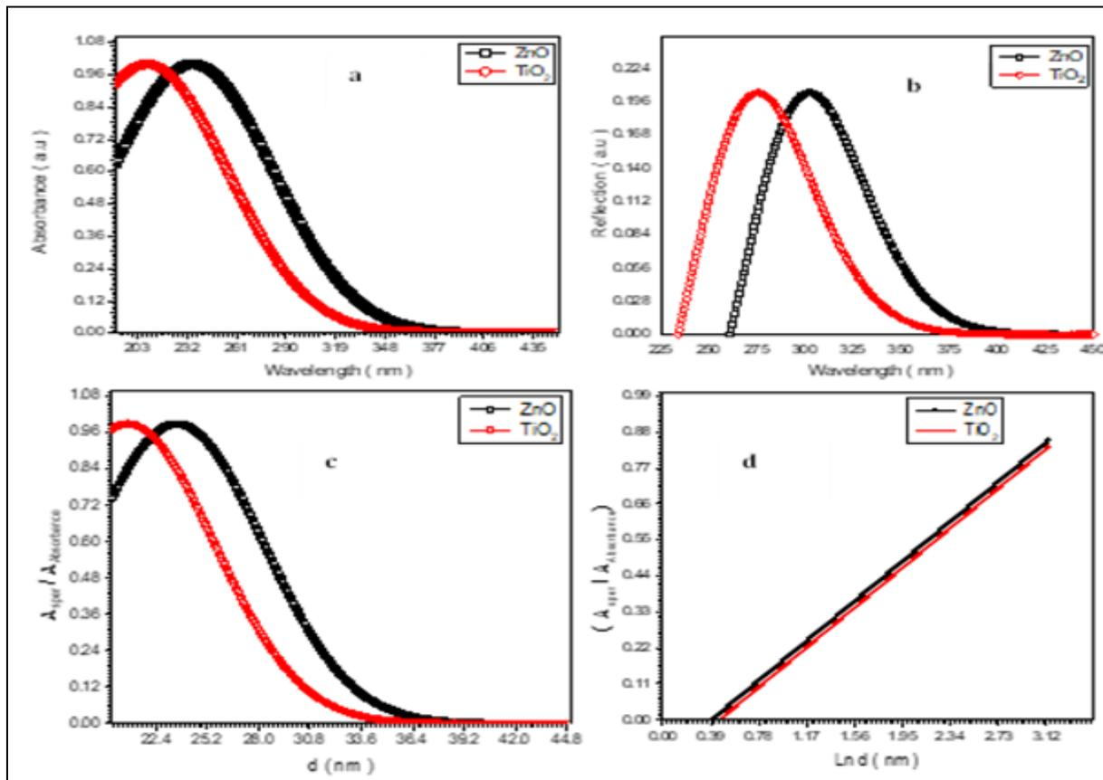
Fig. 3: Calculated particle size of ZnO and TiO<sub>2</sub> nanoparticles by optical method
