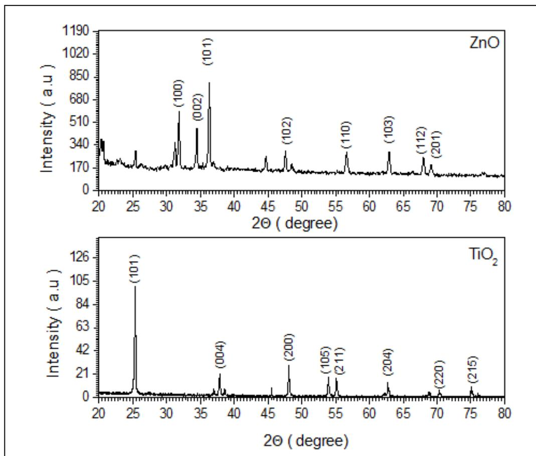
Fig. 1: XRD Pattern of (ZnO and  $\text{TiO}_2$ ) nanoparticles
