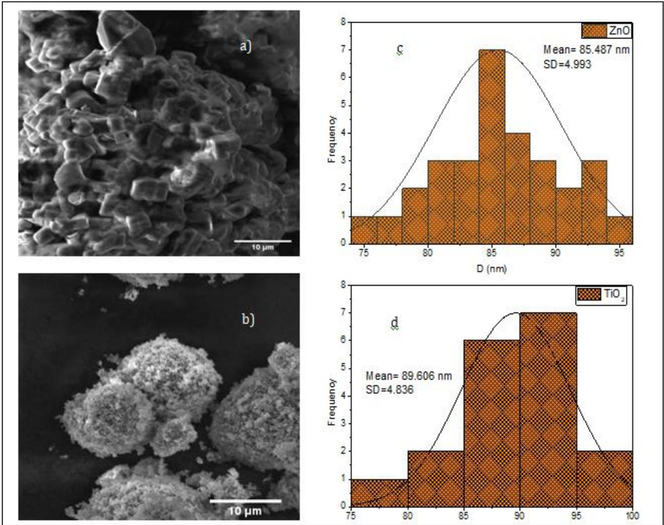
Fig. 2: SEM images (a, b) and particles size distribution (c, d) of (ZnO and TiO<sub>2</sub>) nanoparticles
