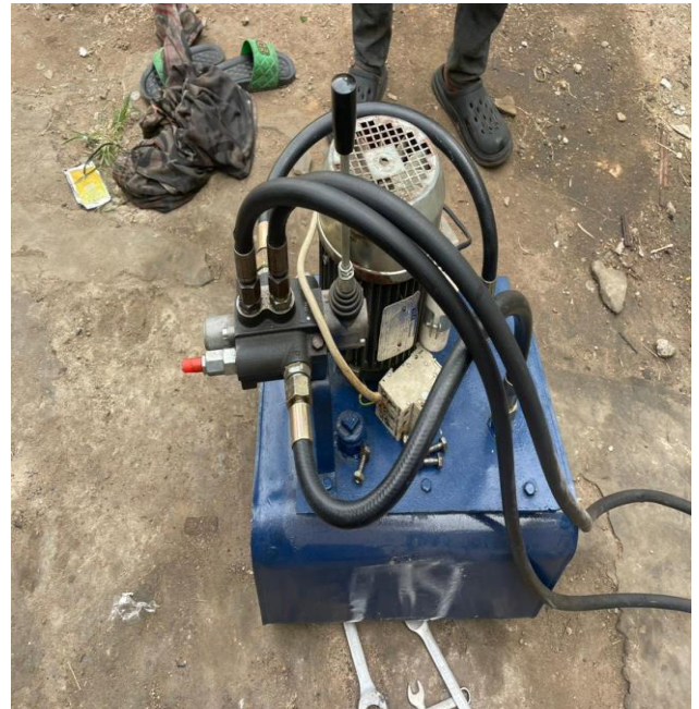
Fig 6: Electric motor with hydraulic tank and control valve
