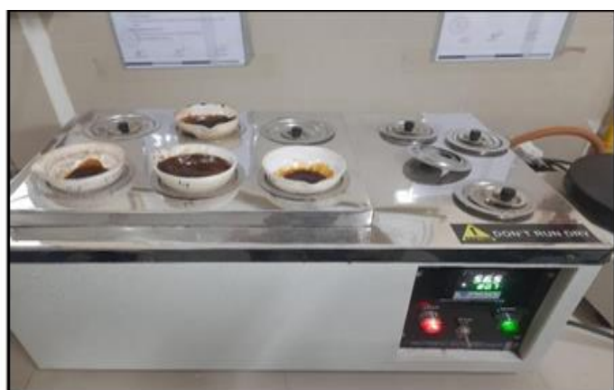
Fig. 8: Evaporation of solvent from extract of sample on steam water bath at 110°C
