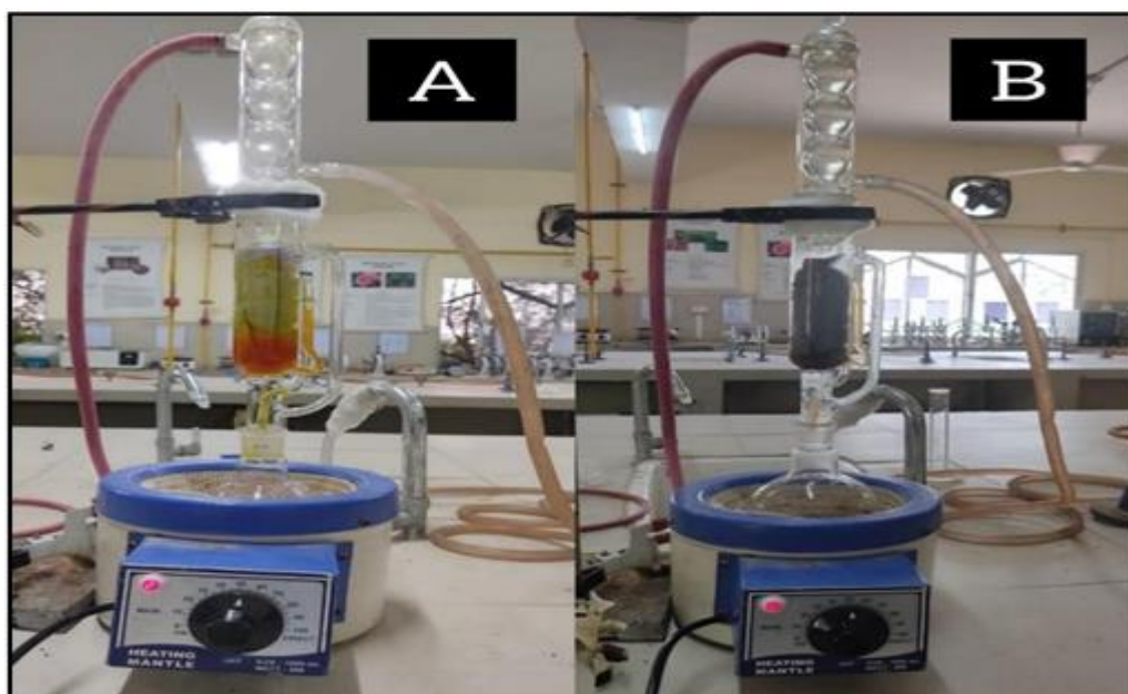
Fig. 9: A) Soxhlet extraction assembly for extraction curcumin from Turmeric and B) Soxhlet extraction assembly for Nigella sativa
