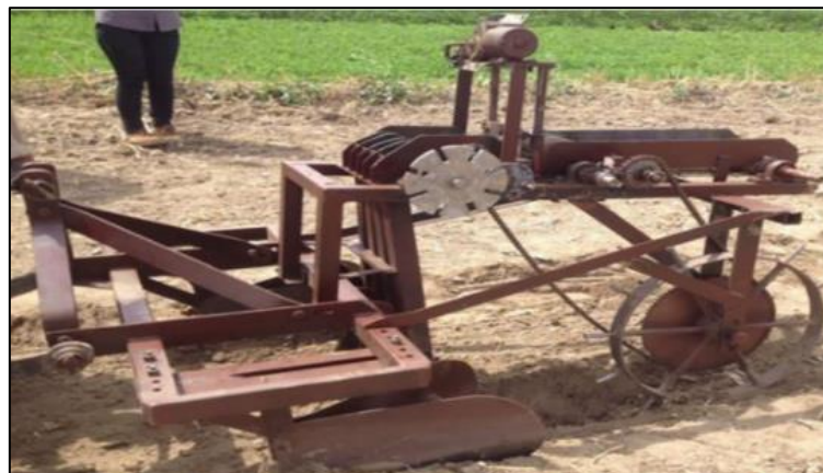
Fig 4 Side View of the Developed Onion Trans planter (Kumawat L. 2020)
