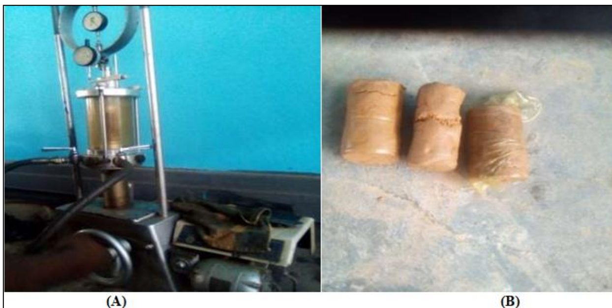
Plate 1: Fly Ash Modified Lateritic Soil During and after Triaxial Test
