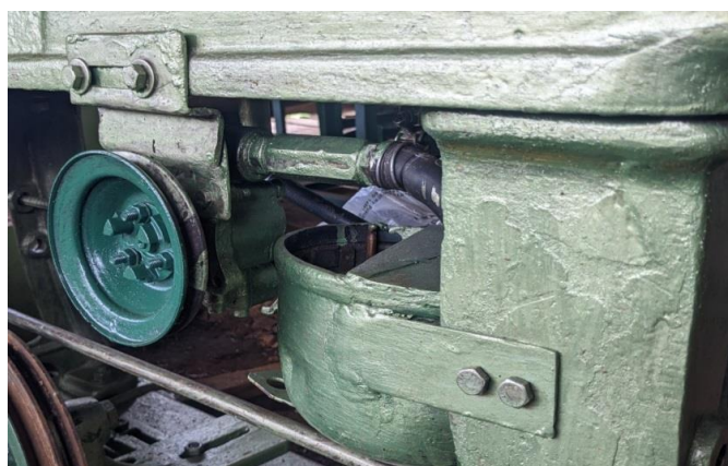
Fig 15 Pump and Tank of the Cooling System
