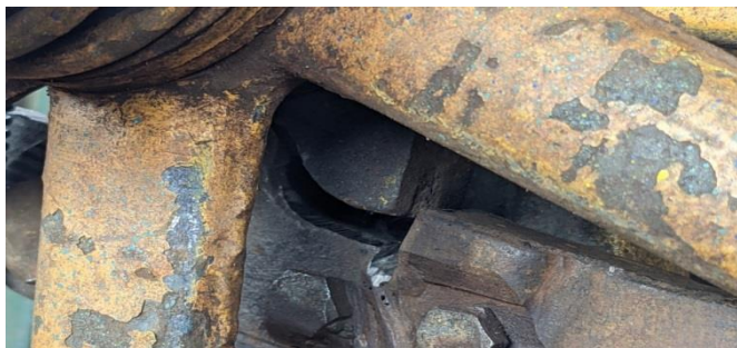
Fig 6 Picture of the Clutch Lever and Trip Lever before Corrective Action
