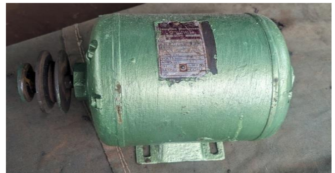
Fig 17 Motor after Corrective Maintenance
