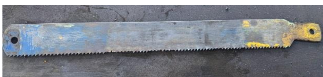
Fig 7 Worn out Blade
