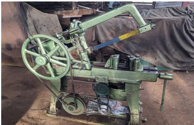
Fig 19 Power Hacksaw after Implementing Corrective Actions
