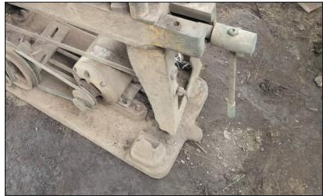
Fig 8 Picture of Broken Legs of the Power Hacksaw Stand
