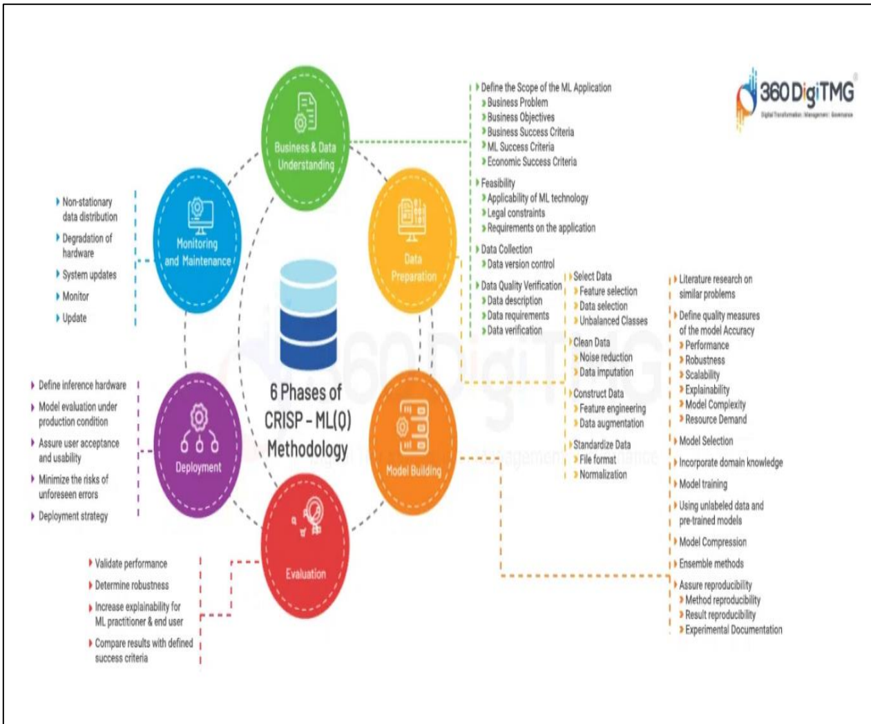
Fig. 1: CRISP-ML (Q) Methodological Framework, Outlining its Key Components and Steps Visually. (Source:-Mind Map - 360digitmg)
