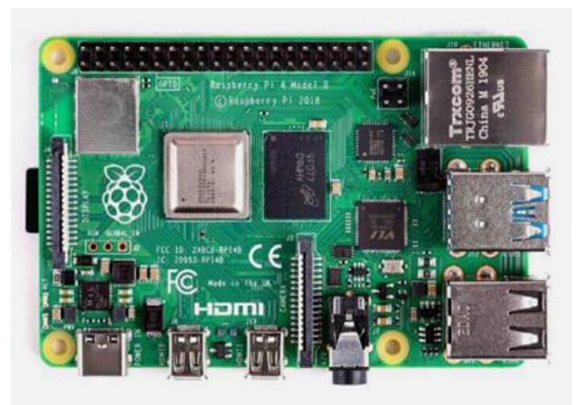
Fig 2. Raspberry 8GB Raspberry Pi 4 Model B RAM Quad core 64-bit 1.5GHz
