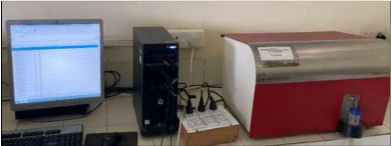
Fig. 1: Instruments used for Somatic Cell Count, DELTA Instrument, BV Kelvinlaan 3,9207 JB Drachten, The Netherland used for Somatic Cell Count
