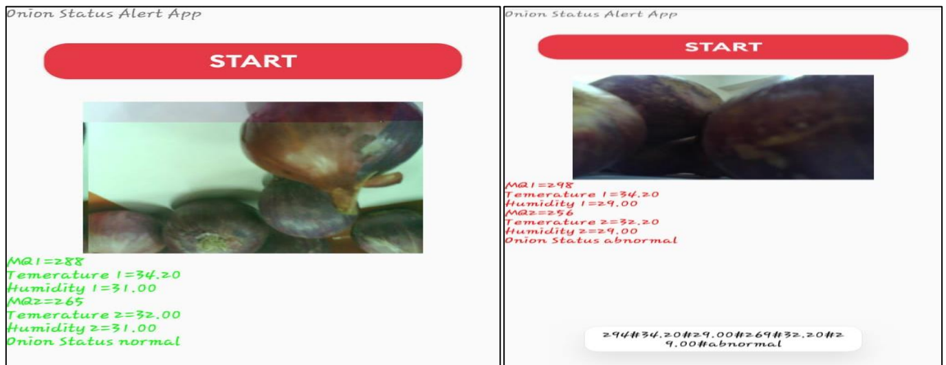
Fig 7: Mobile Alert System (Green – Normal, Red – Abnormal)
