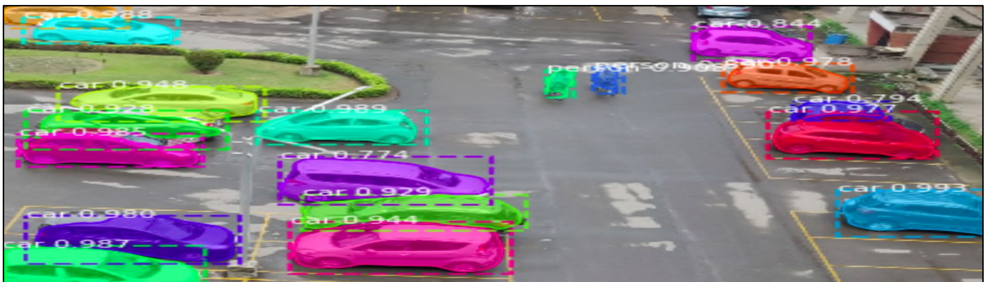
Fig 16: Output of Mask R-CNN Algorithm at Parking Area
