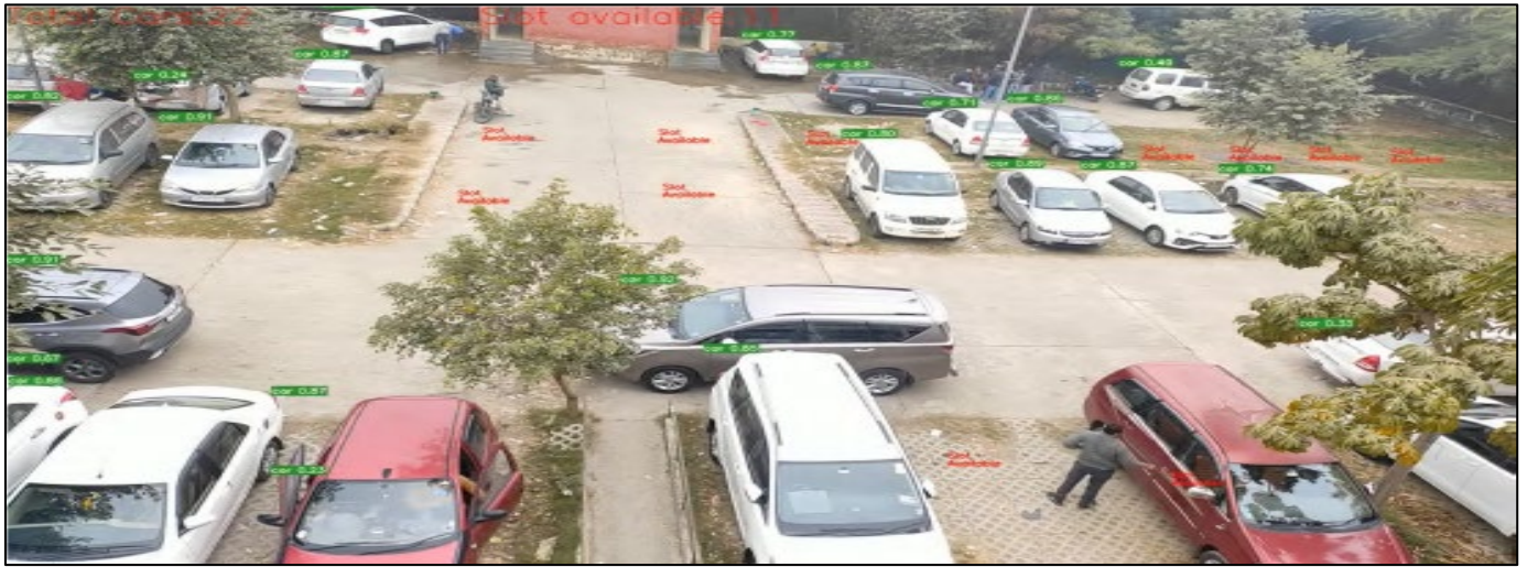
Fig 28: YOLOv5 based Parking Occupancy Detection System
