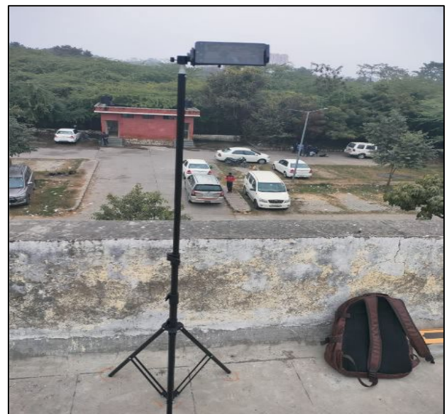
Fig 20: Camera Setup on the Roof of the Building
