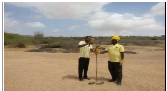
Fig 5: Measuring Cadaadley Riverbed by using Iron Rod(2m) to Identify Depth of Impermeable Layer in the Riverbed.
