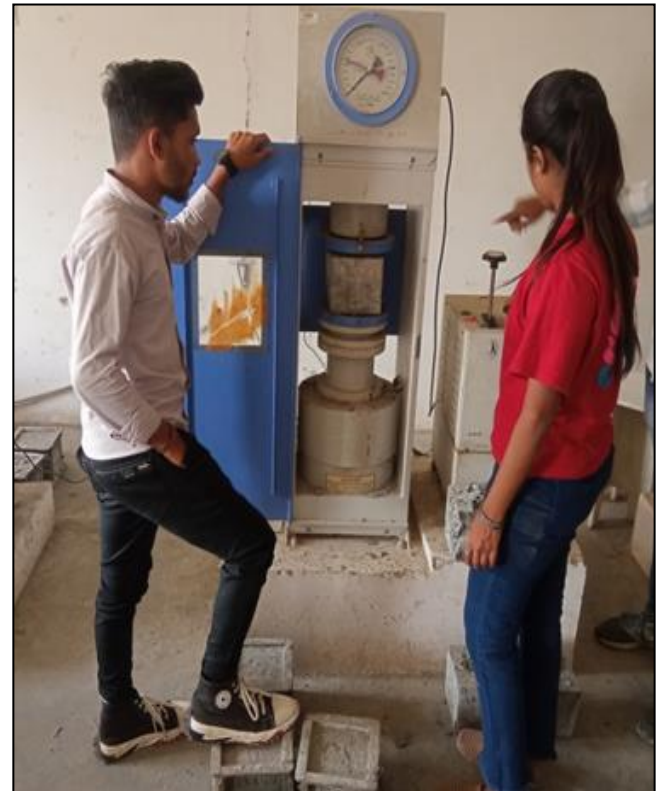
Fig 5: Compressive Strength Test of Cube
