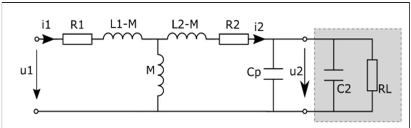
Fig 2 ECD of Magnetic Coupled RFID Reader Coil and Transponder Coil
