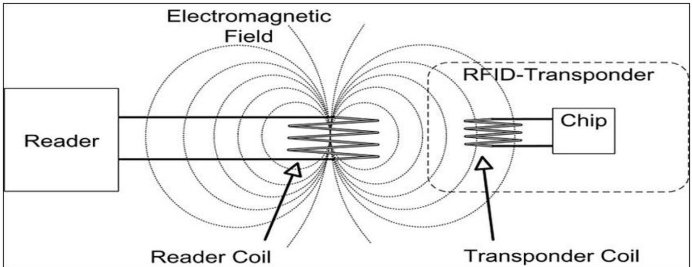
Fig 1 Inductive Coupling of RFID
