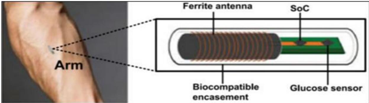
Fig 5 Implanted Glucose Detection Model [1]
