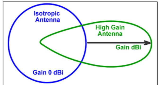
Fig 4 Antenna Gain
