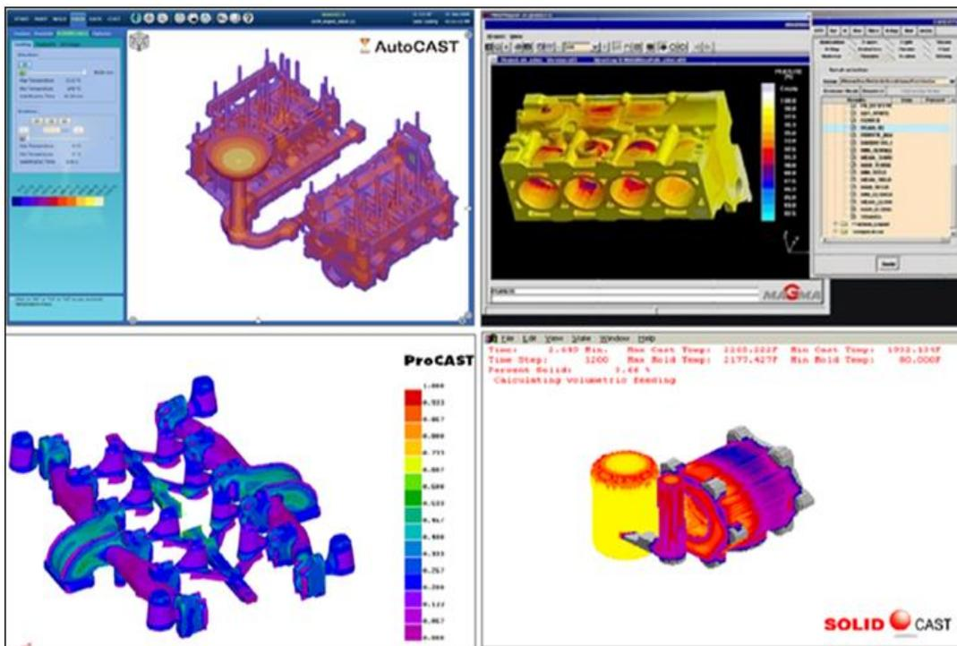
Fig 3 Popular Casting Simulation Software (Auto CAST, MAGMA, Pro CAST, and Solid CAST) user Interface
