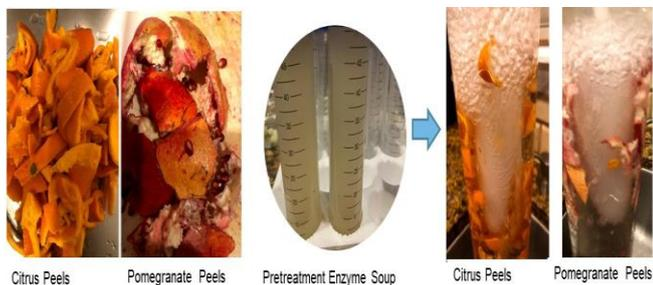
**Fig 3.** Treatment of citrus and pomegranate peels with enzyme mix in the airlift bioreactor.
