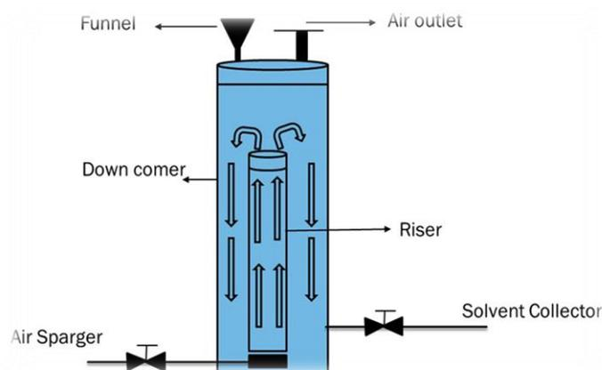
**Fig.1.** Airlift bioreactor design for enzymatic treatment and extraction of antiviral bioactives from Fruit peels.
