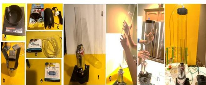
**Fig 2.** Materials (a-e) used in making airlift bioreactor for the extraction of the bioactive from fruit peels. The reactor was built (f-i) as per the design mentioned in Fig 1.
