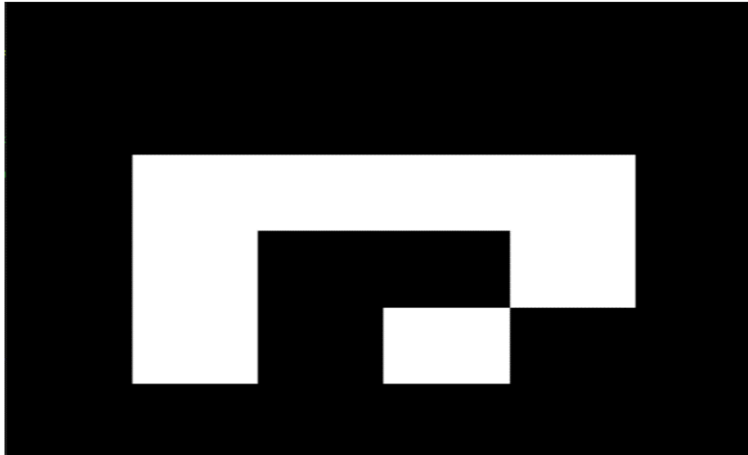
Fig. 8: Aruco Marker for Precision Landing
