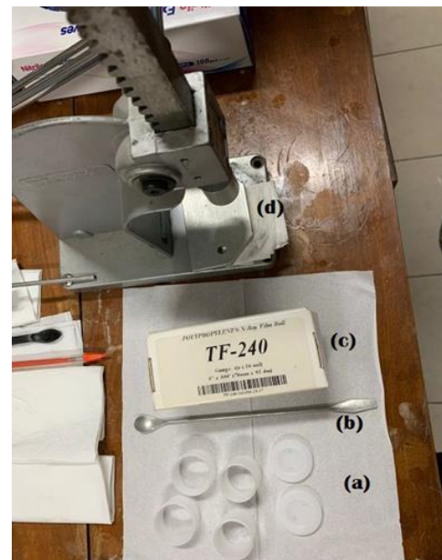
Fig 2 Equipment for XRF Test; (a) Sample Cup Sets, (b) a Stainless Spatula, (c) a Thin Film, and (d) a Press Tool.
