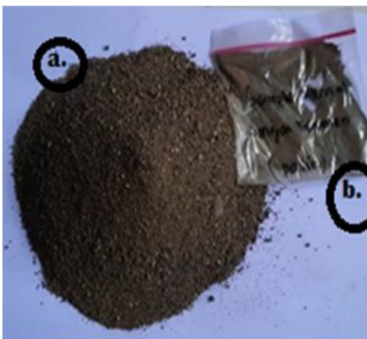
Fig 1 Sample (a) Sand of Alluvial Gold in Kebakalan, and (b) Samples with a Particle Size Fraction of -100 Mesh in a Plastic Bag.
