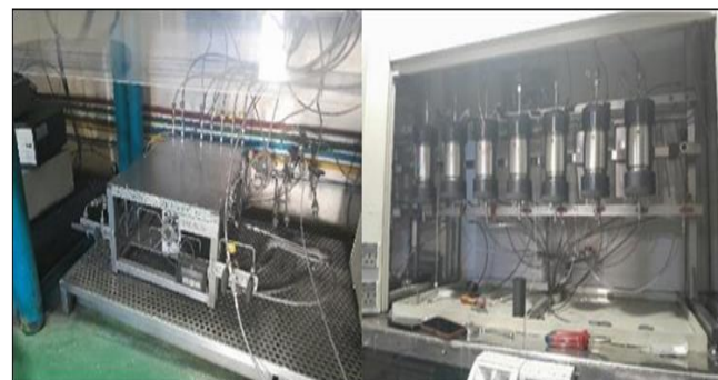
Fig 5 Cement Plug Cleaning Machine/Hydrostatic Core Holder
