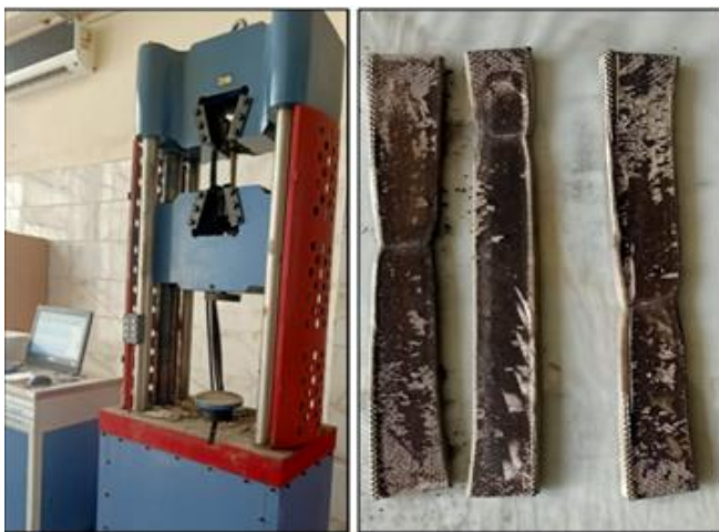
Fig 2 Tensile Coupon Machine and Typical Failure Mode.
