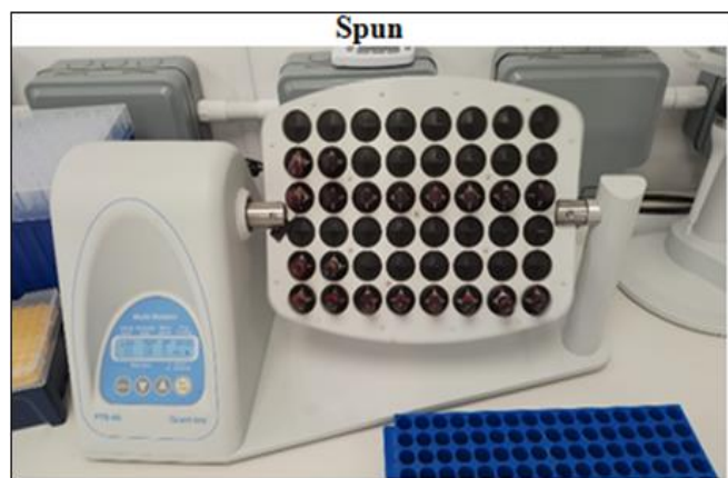
Fig 2 The Samples were Spun in a Rotator. this helps in the Immersion of the Cell Suspension.
