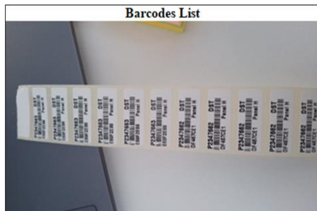
Fig 3 This Barcode was Generated Unique to each Sample. the Barcodes were Scanned to Enter the Sample Number into the Reader to Link the Strip to the Sample Number in the Reader.
