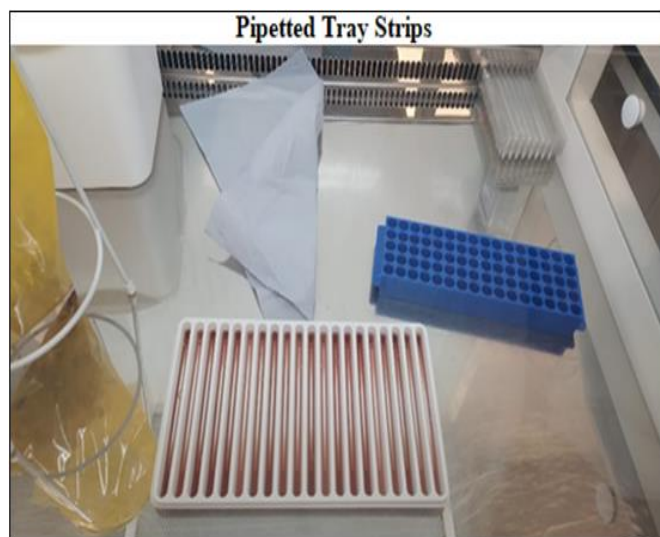
Fig 6 The Samples were Pipetted into the Tray with the Respective Strip
