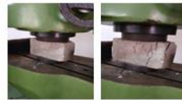
Fig 4 Compressive Strength Test in UTM
