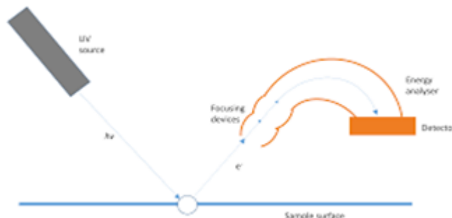
Fig 16 Principle of UV PES
