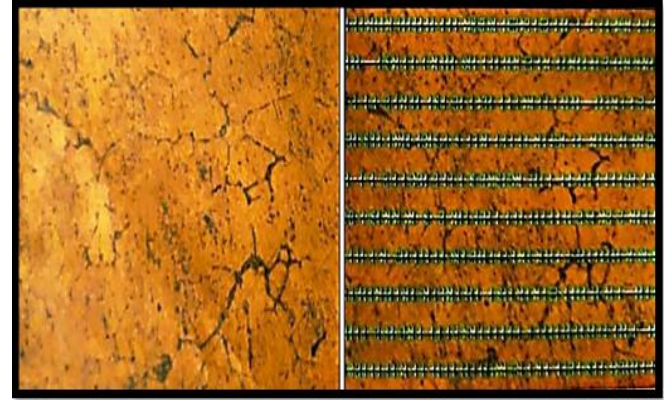
Fig 24 Metallurgical Microscopy (10µm) of Aluminium 6061- 1.2%GNP
