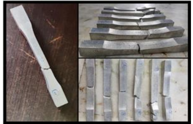
Fig 7 Specimen tested by UTM
