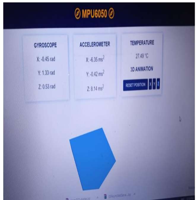
Fig 15 The Gyroscope Sensor Showing the Position of the Generator Set During Testing
