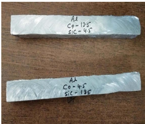
Fig 1 Specimen for Tensile & Impact Test
