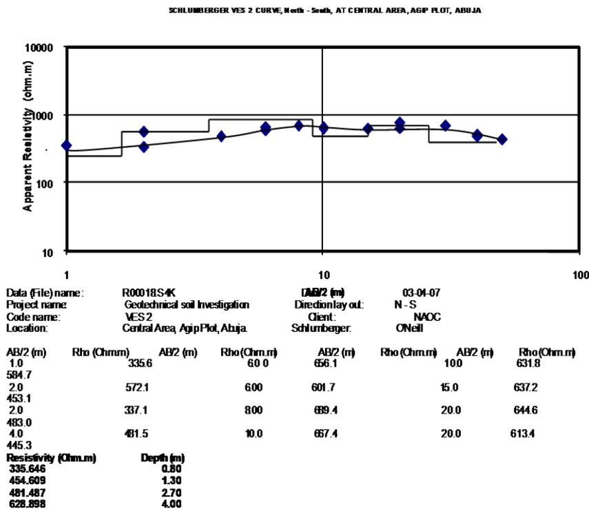
Fig. 4: Geo-electric soil data for Direction X at Abuja site
