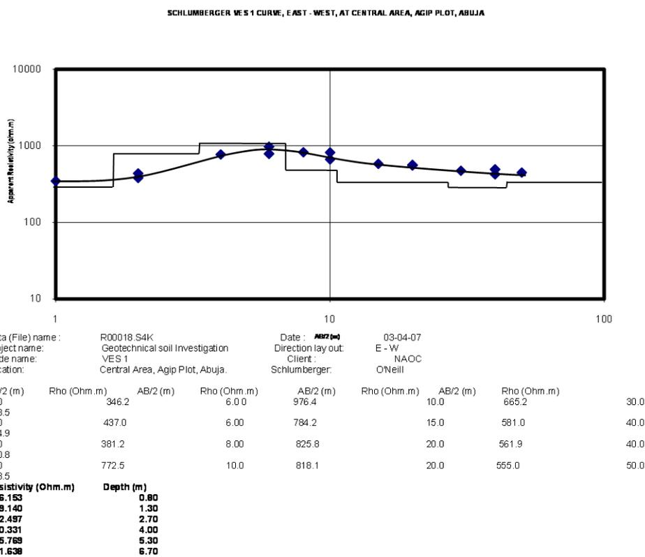
Fig. 5: Geo-electric soil data for Direction Y at Abuja site
