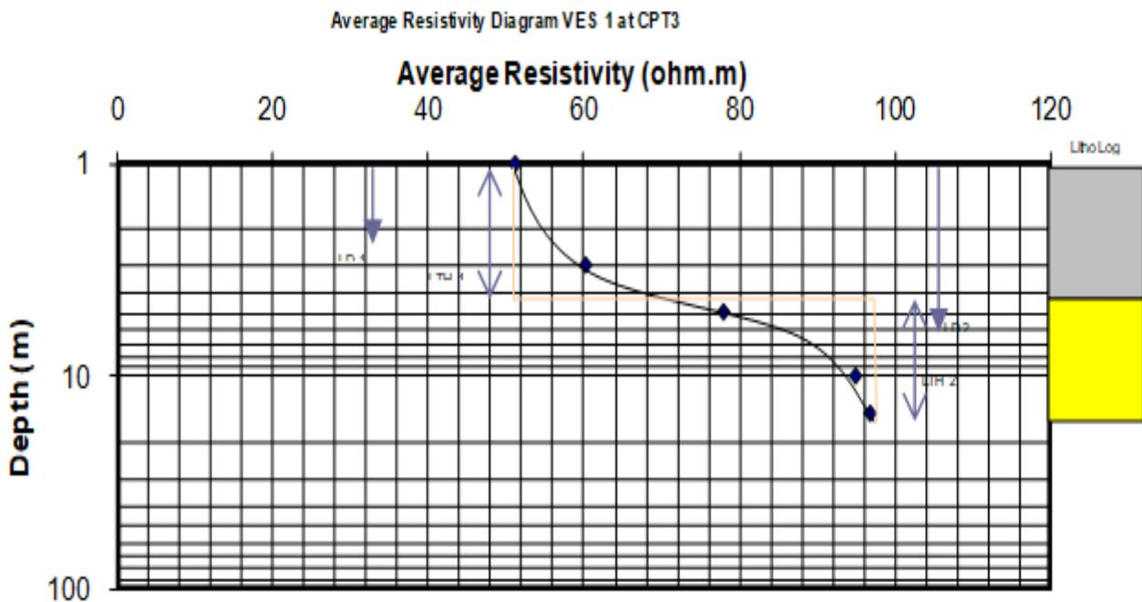
Fig. 2: Geo-electric ground model of VES1 at CPT3 location at Oguta
