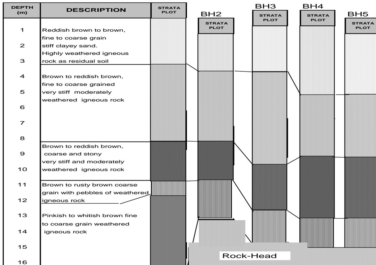
Fig. 6: Composite Soil Profile at a Weathered rock area in Abuja, Nigeria
