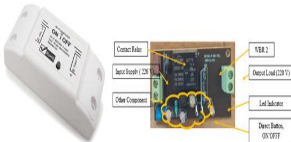
Fig. 1: Smart Breaker AI-BR01 & Construction of Smart Breaker AI-BR01
