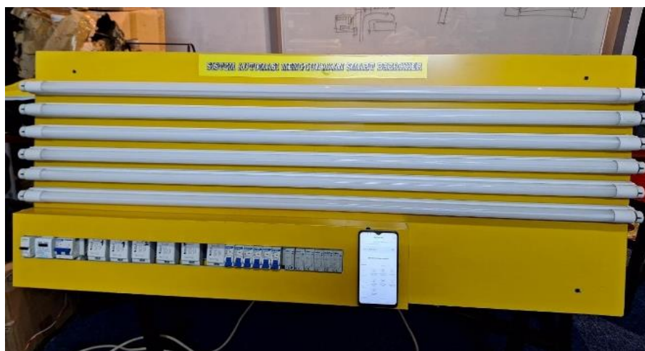
Fig. 5: Automation System with Smart Breaker
