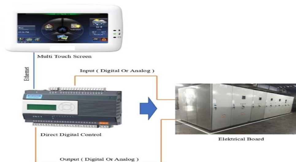
Fig. 1: Schema Building Automation System at Building
