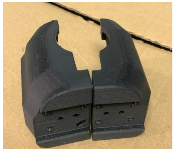
Fig 1. Jaw Gripper Made of Onyx-Carbon Fiber Reinforced
