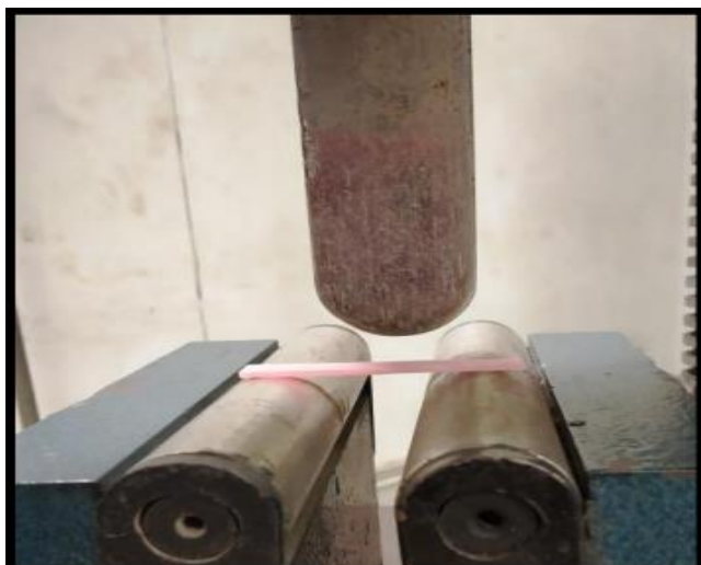
Fig 7 Testing of Flexural Strength on Universal Testing Machine
