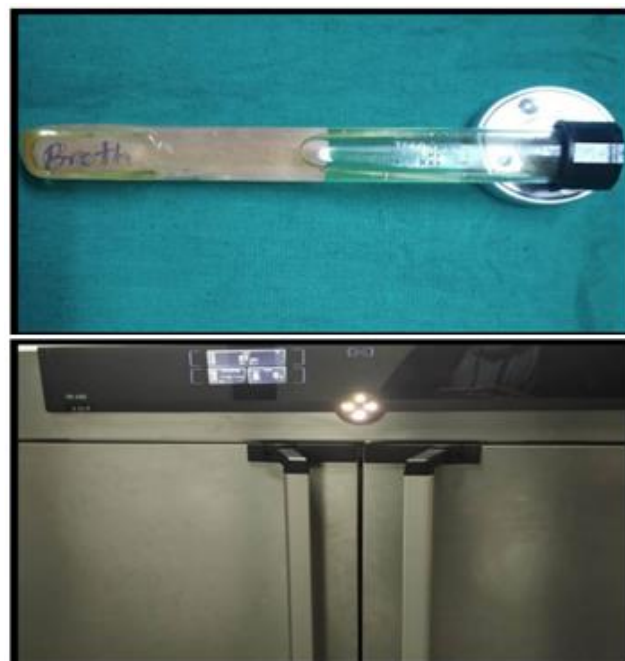
Fig 9&10 Specimens Immersed in BHI Broth Containing Microbial Strains & Incubated at 37° C
