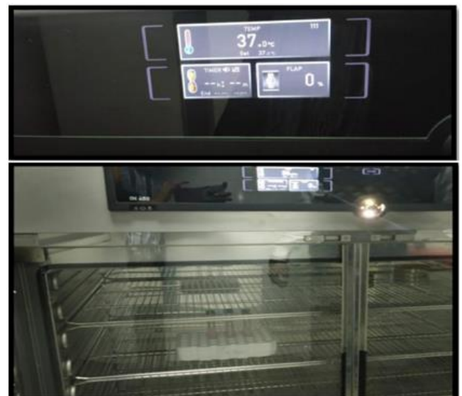
Fig 6 A&B Specimens Immersed in DistilledWater Placed in Incubator at 37° C
