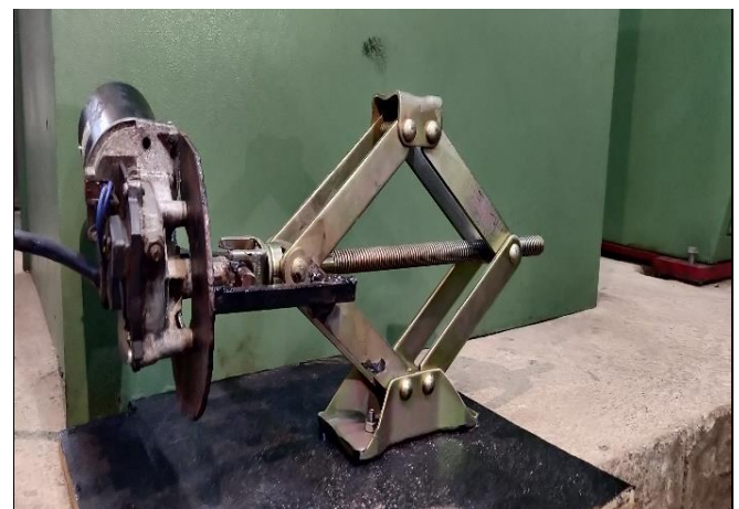
Fig 5 Prototype of Motorised Scissor Jack
