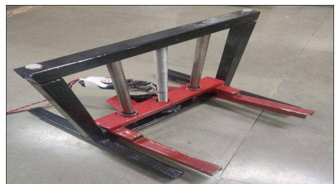
Fig 6 Prototype of Motorised Screw Jack
