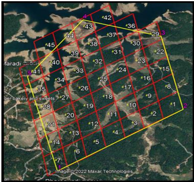
Fig 3 Grids are Created Parallel to 1 st and 2 nd Sides of the Polygon
