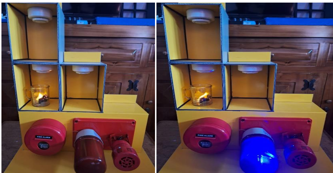
Fig. 9: Condition At Room 1-GF, Detector is On and Announcement On
