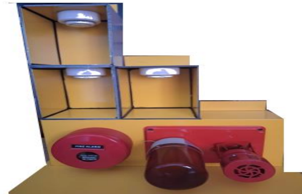
Fig. 8: Actual Illustration Of Fire Alarm System
