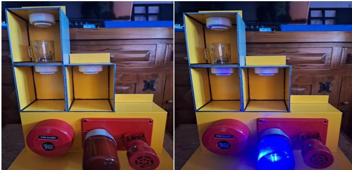
Fig. 11: Condition At Room 1-2ND, Detector is On an Announcement On
