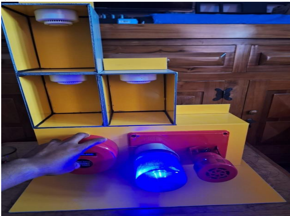
Fig. 12: Manual Call Point Is On an Announcement On
