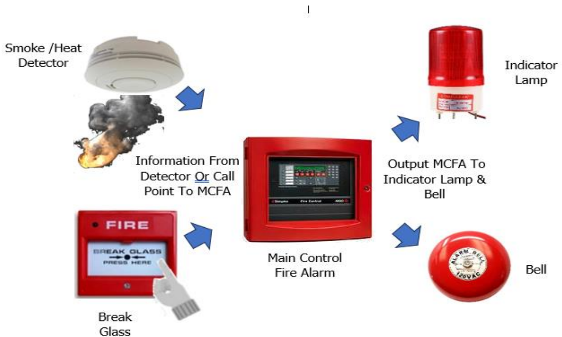
Fig. 4: Fire alarm system duty cycle
