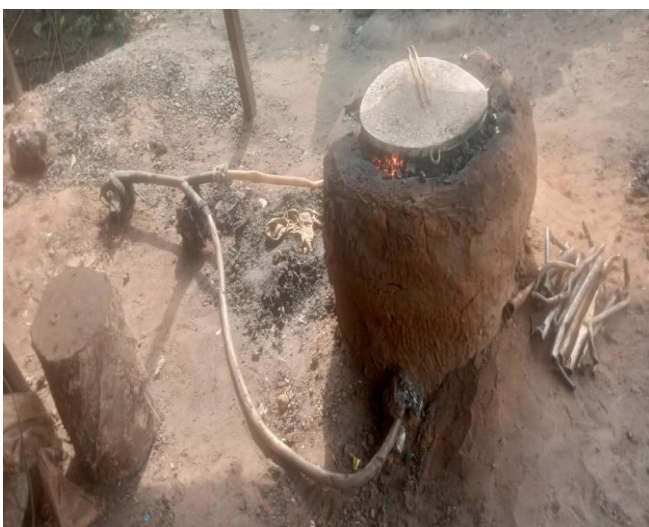
Plate III An Electrically Charged Funnel for Smelting the Metals are being Heated for Casting
