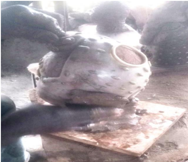
Plate 1 Detailed Wax being Covered with Red Sand at Aigbes Foundry
