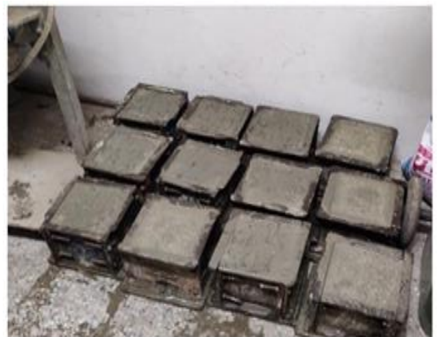
Fig 1 All the Moulds are filled with Concrete
