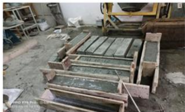
Fig 4 RCC Beam kept for Curing
