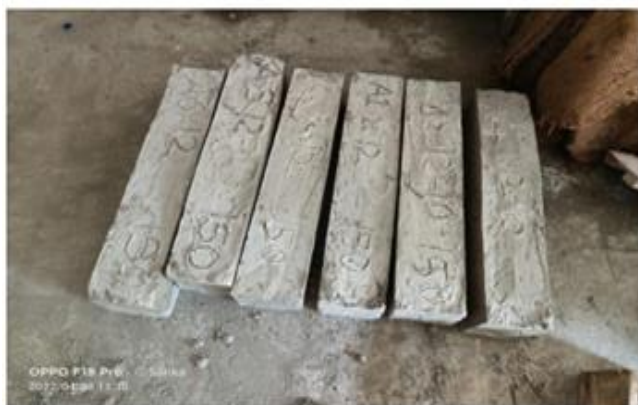
Fig 5 Beam kept for Curing
