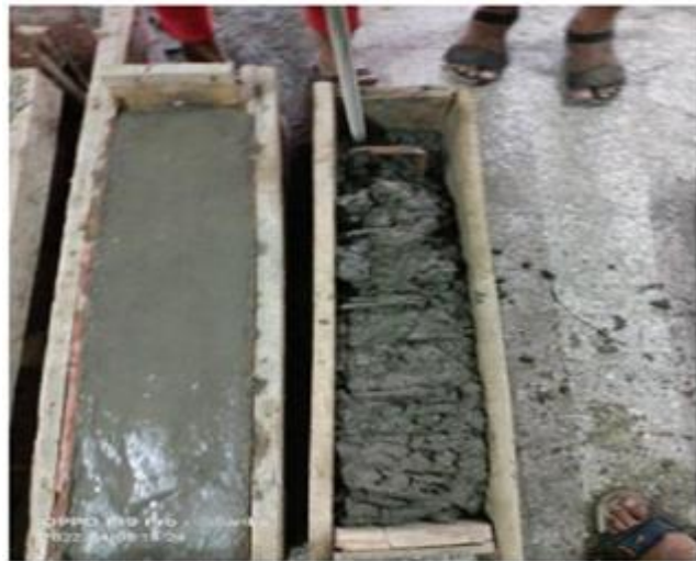
Fig 3 RCC Beam Filled
