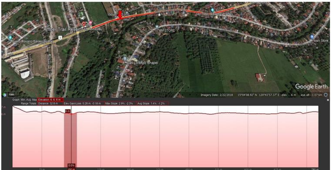
Fig 18 Slope Elevation with Catchment Area 1
