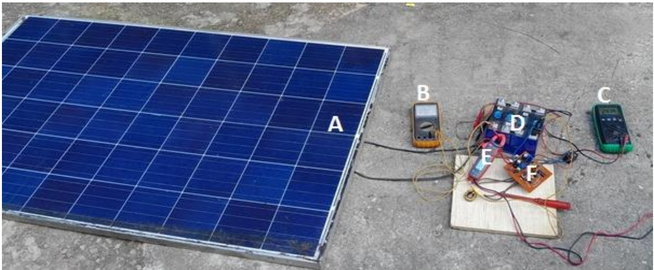
Fig 21 The System test setup, (A) 260W Solar panel (B) Battery voltmeter (C) PV Voltmeter (D) Test Battery (E) PV Current meter (F) MPPT Board under test.
