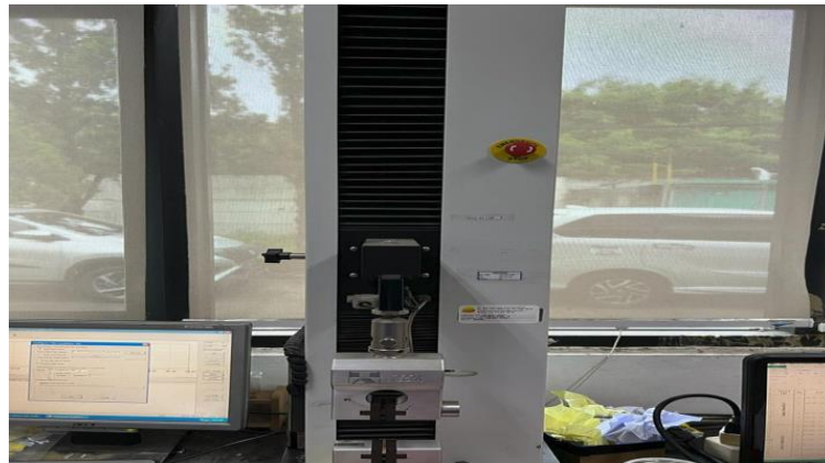
Fig. 2: EJA Series Twing-Albert Tensile Testing Machine
