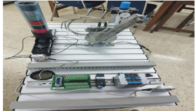
Fig 2 MPS Distribution Station [8]
