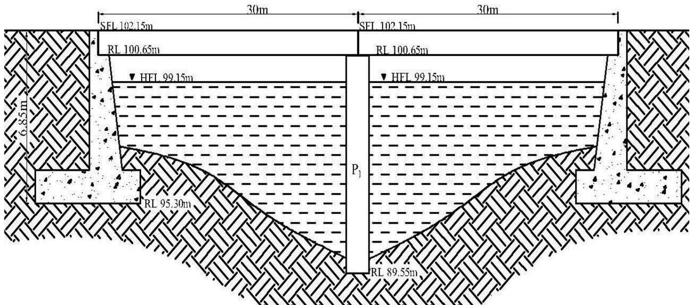
Fig 3.15 Typical Bridge Section with the Span of 30m
