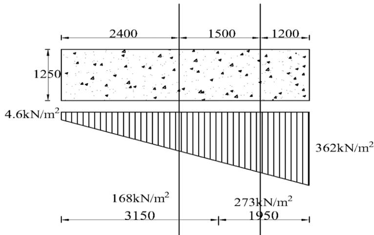
Fig 4.4 Abutment Base Moment Diagram
