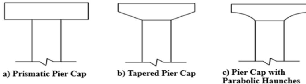
Fig 2.22 Different Types of Pier Caps for Single Column Piers (FHWA, 2012)
