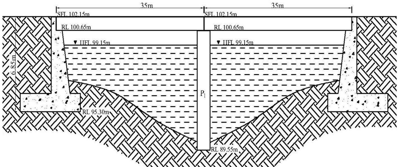
Fig 3.17 Typical Bridge Section with the Span of 35m
