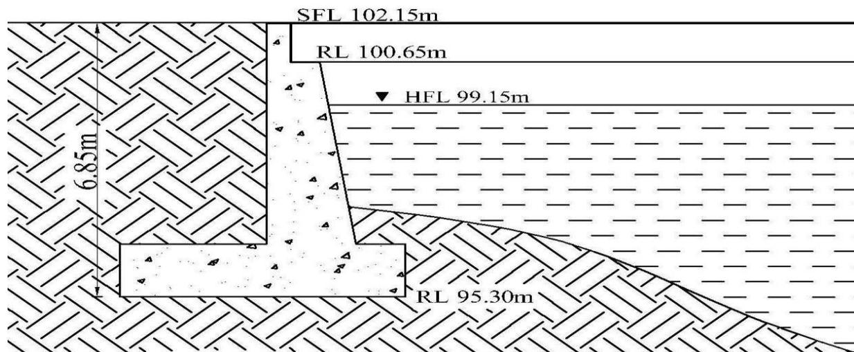
Fig 3.6 Schematic Diagram of the Abutment
