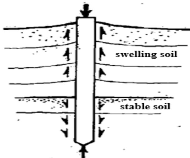
Fig 2.5 Piles in Expansive Soils can Control Seasonal Movements (Patel, 2012)
