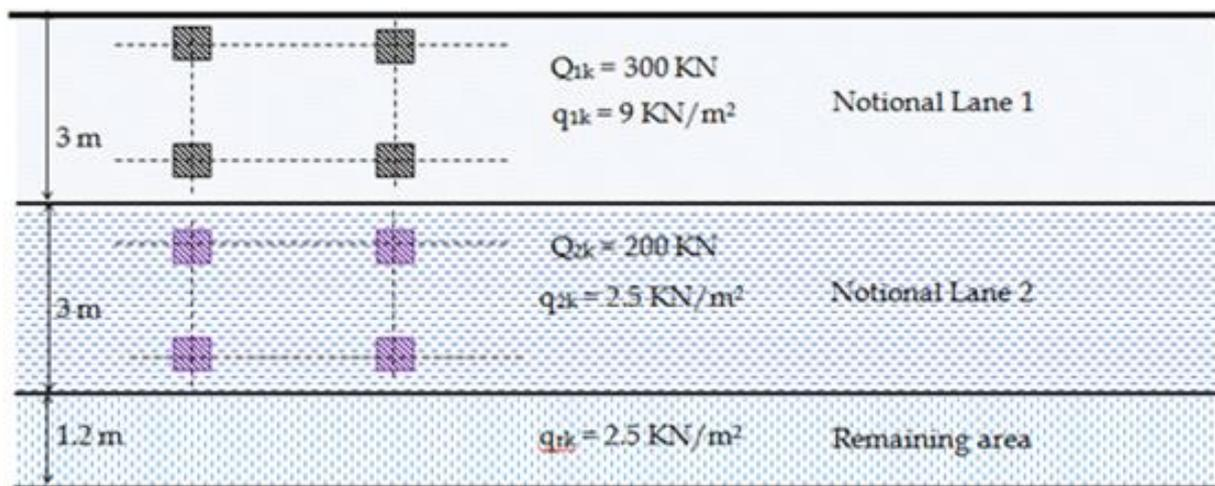
Fig 3.3 Application of Load Model 1, on a Deck with Two Notional Lanes
