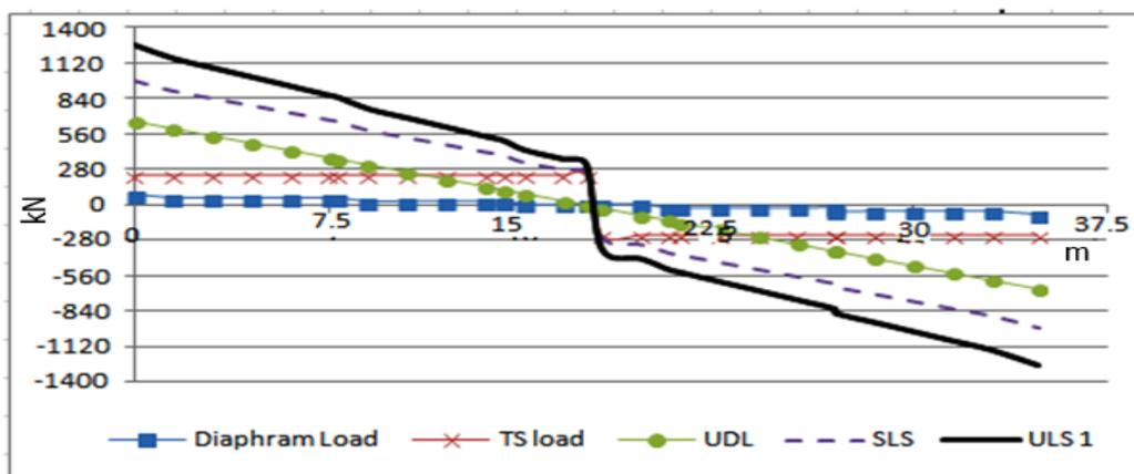
Fig 4.11 Shear Force Diagram of Span 35m
