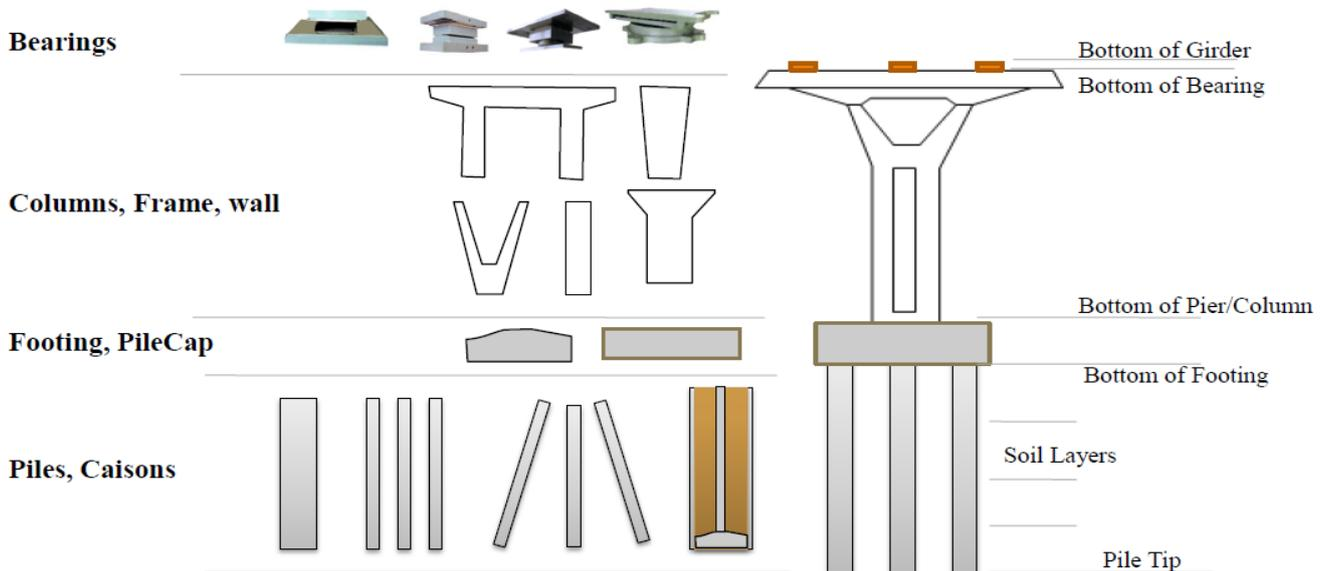
Fig 2.25 Subcomponents of Typical Bents (Anwar, 2015)
