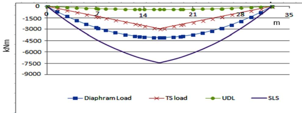
Fig 4.9 Moment Diagram of Span 30m
