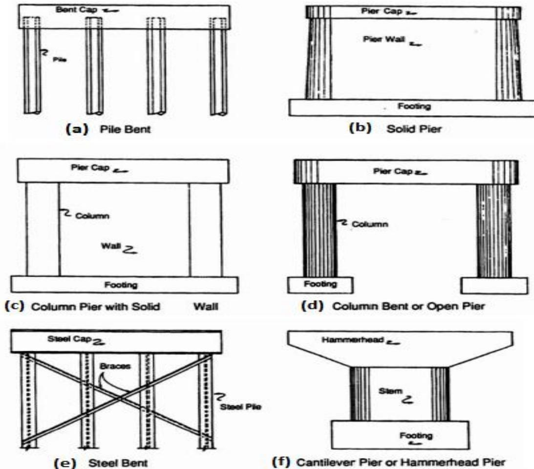
Fig 2.20 Pier Bent types (Anwar, 2015)
