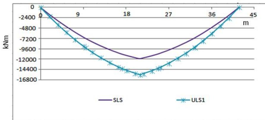
Fig 4.32 Moment at Middle of the Beam for First Combination Diagram of Span 40m
