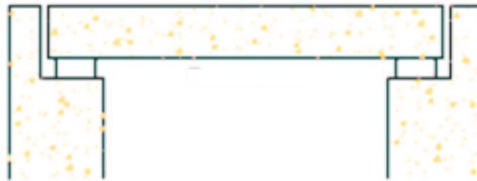
Fig 2.15 Both Abutments with Elastomeric Bearings only (Childs, 2015)
