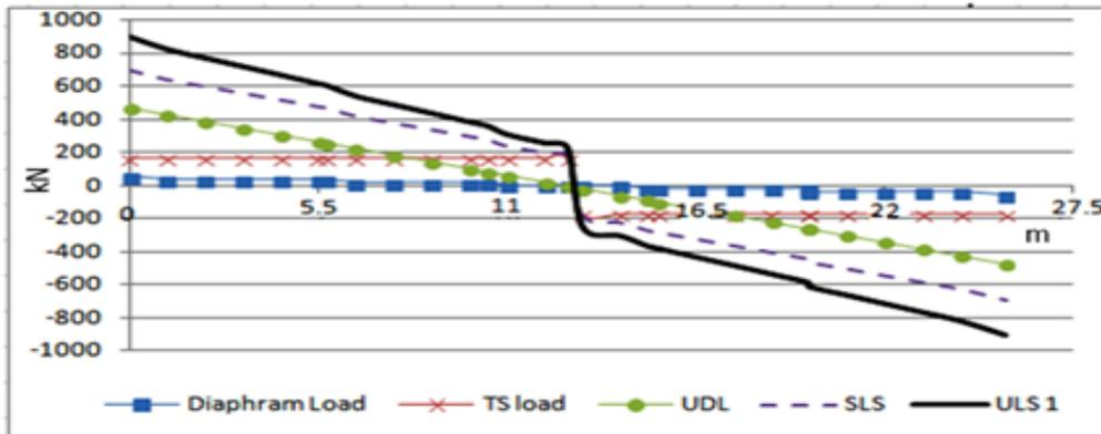
Fig 4.21 Shear Force Diagram of Span 25m
