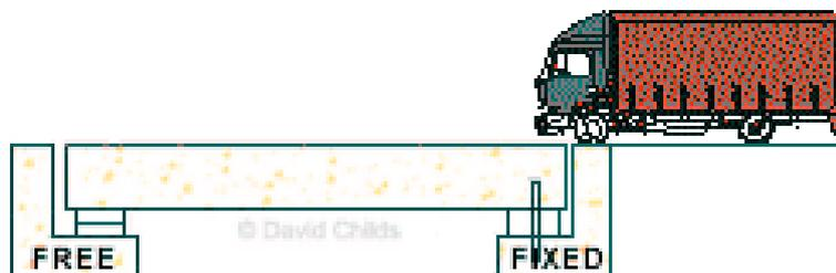
Figure 2.17 Free Abutment with Sliding or Elastomeric Bearings (Childs, 2015)
