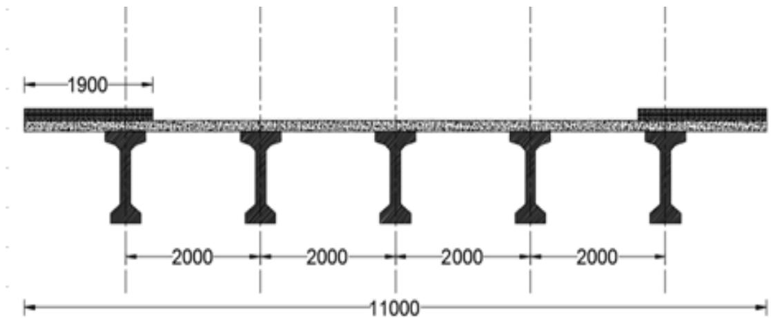
Fig 3.2 Cross Section of Bridge Deck Diaphragms (Cross-Girders) Arrangement
