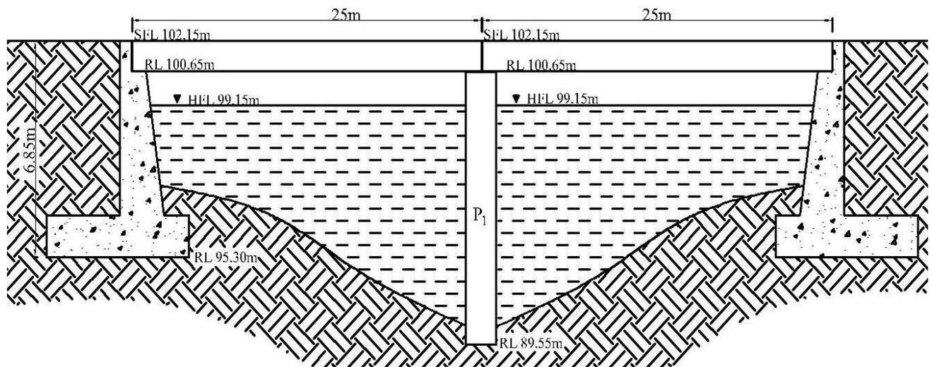
Fig 3.13 Typical Bridge Section with the Span of 25m
