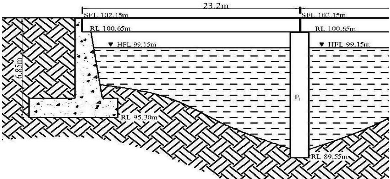
Fig 3.9 Pier Position on Bridge Span of 23.2m
