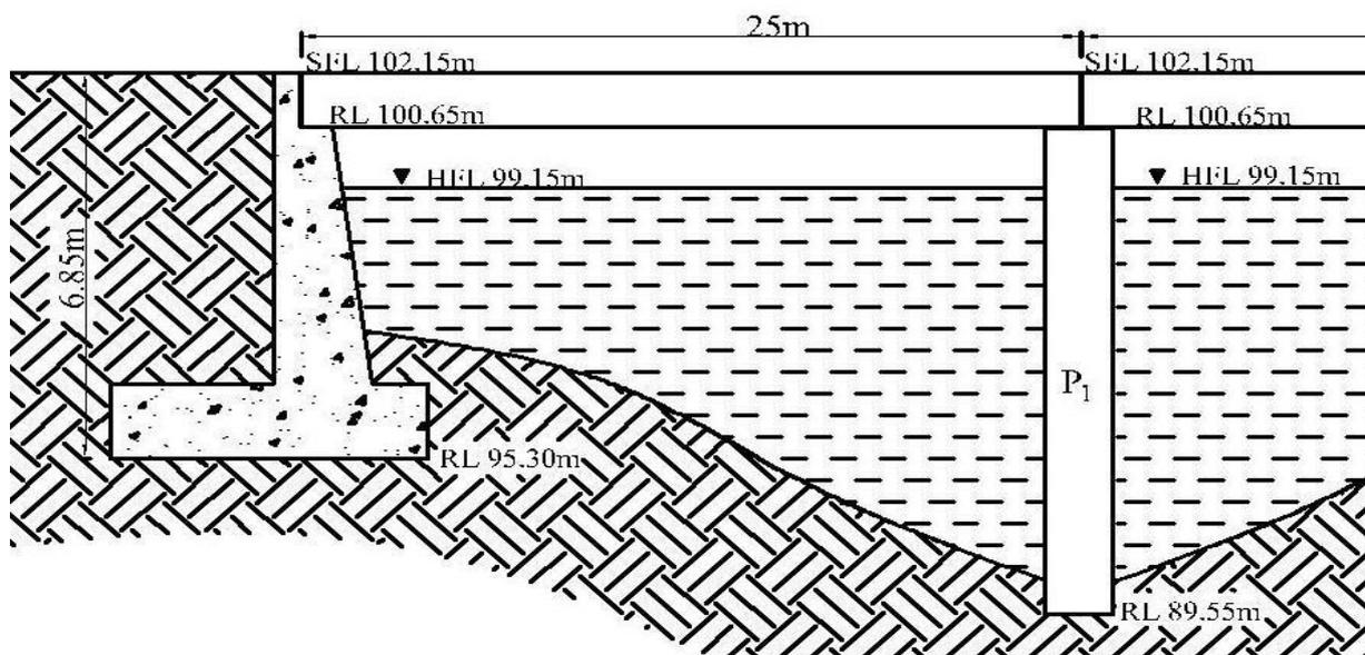
Fig 3.14 Pier Position on Bridge Span of 25m
