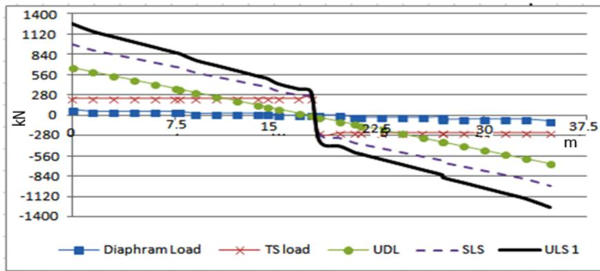
Fig 4.27 Shear Force Diagram of Span 35m
