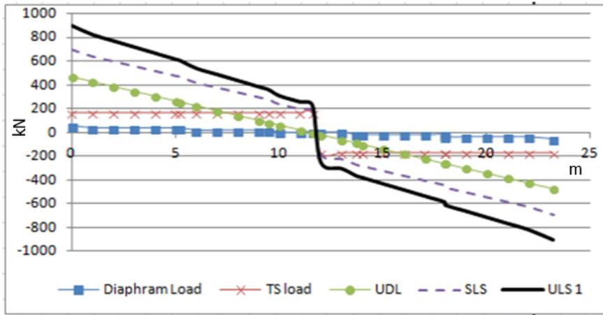
Fig 4.18 Shear Force Diagram of Span 23.2m
