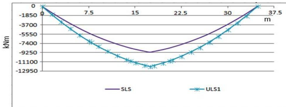
Fig 4.29 Moment at Middle of the Beam for First Combination Diagram of Span 35m
