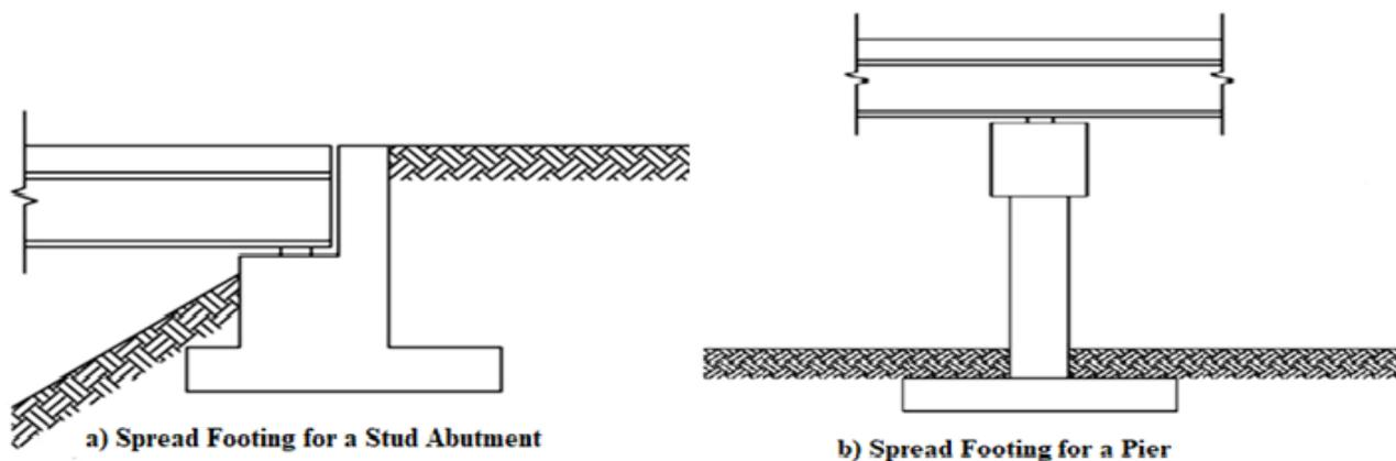
Fig 2.1 Spread Footing Applications (FHWA, 2012)
