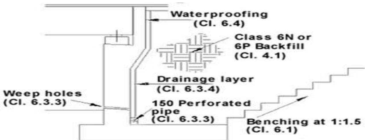
Fig 2.12 Abutment Construction (Departmental Standard BD 30 & Childs, 2015)
