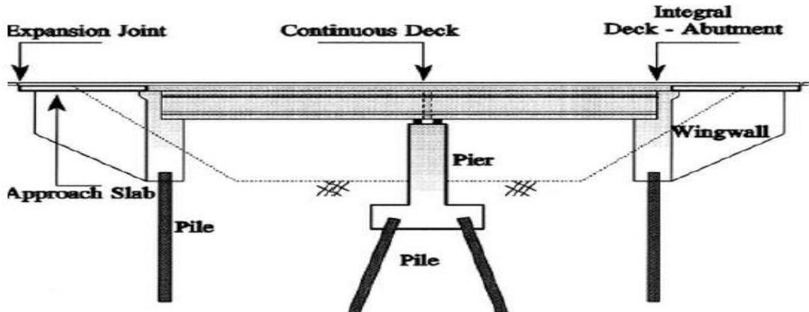
Fig 2.10 Abutment Foundations (Anwar, 2015)
