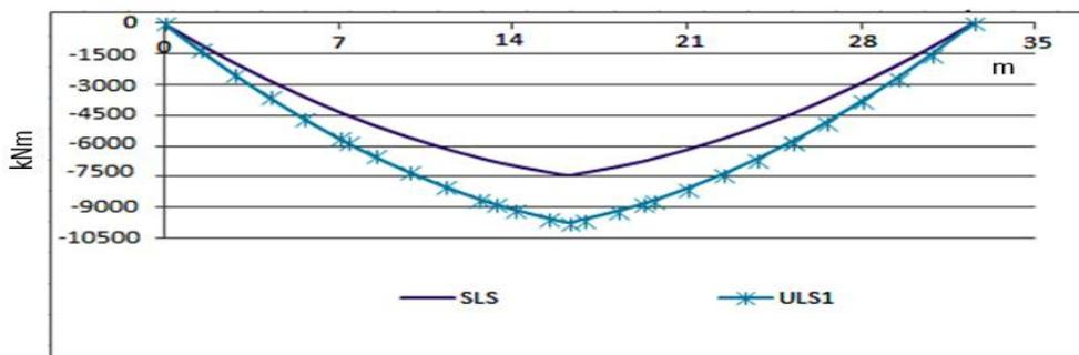
Fig 4.10 Moment Diagram for first Combination of Span 30m
