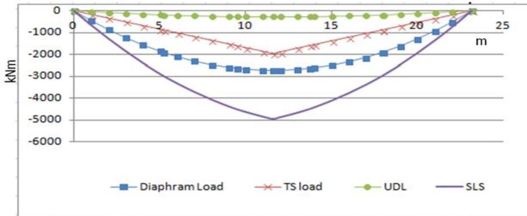
Fig 4.2 Moment Diagram of Span 23.2m
