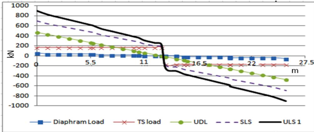
Fig 4.5 Shear force diagram of Span 25m
