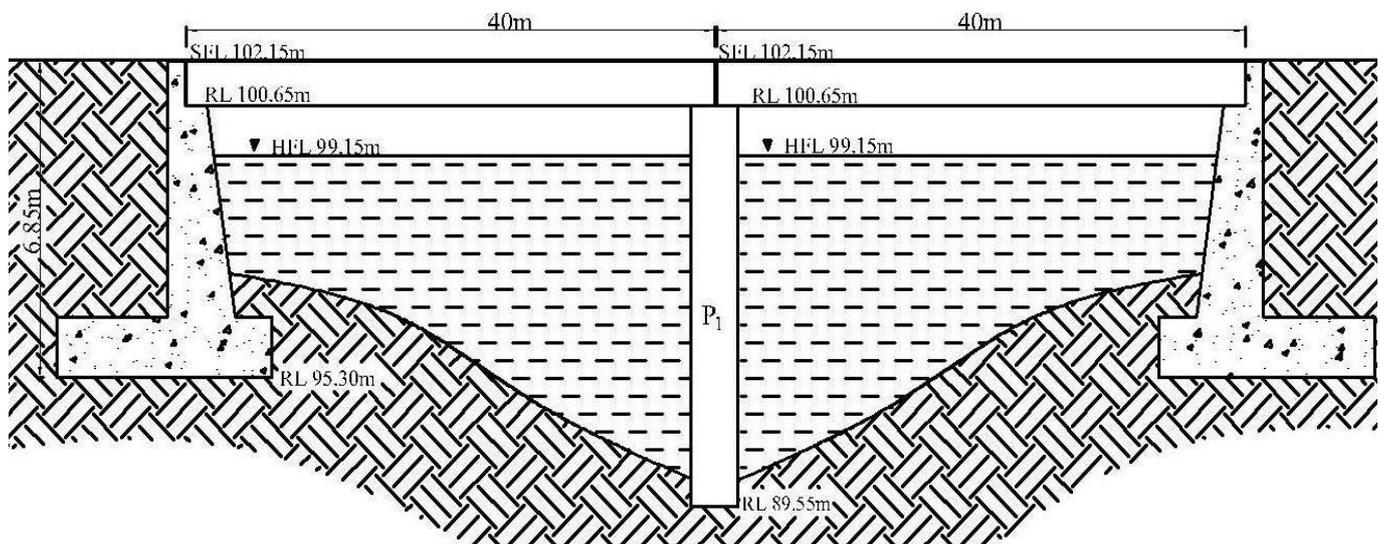
Fig 3.19 Typical Bridge Section with the Span of 40m
