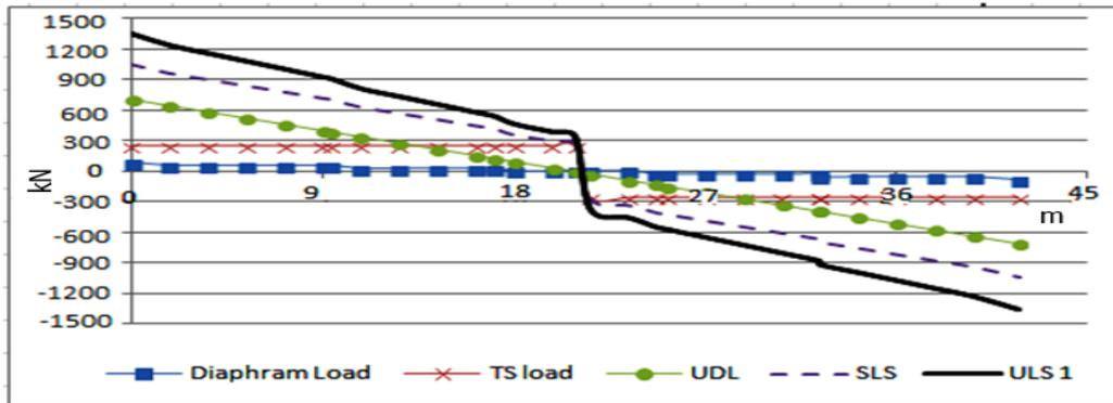
Fig 4.14 Shear Force Diagram of Span 40m
