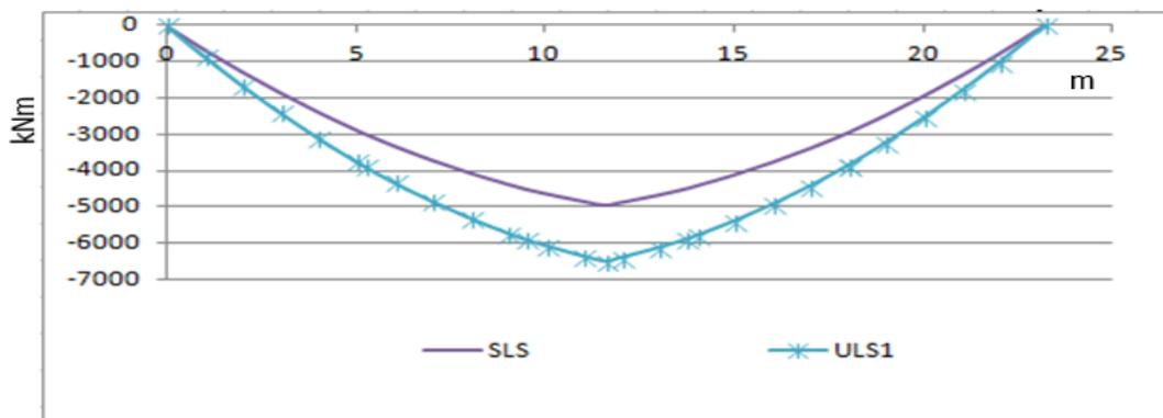
Fig 4.3 Moment at Middle of the Beam for First Combination Diagram of Span 23.2m
