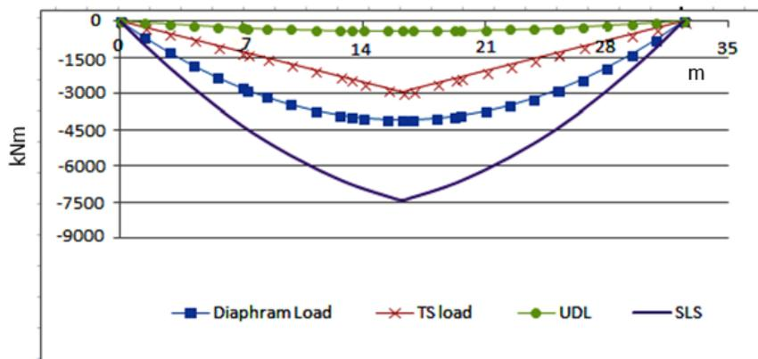
Fig 4.25 Moment Diagram of Span 30m
