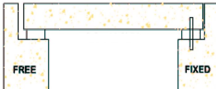
Fig 2.16 Free Abutment with Elastomeric Bearings (Childs, 2015)
