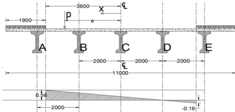
Fig 3.4 Influence Line Diagram of Diaphragms (Cross girders)
