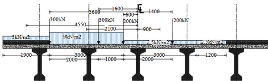
Fig 3.5 Load Model 1: Diaphragms (Cross Girders) Arrangement
