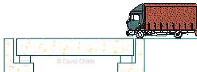
Fig 2.18 Both Abutments with Elastomeric Bearings only (Childs, 2015)
