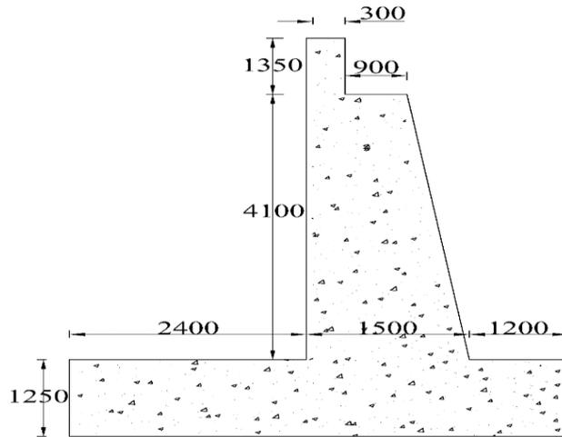
Fig 3.7 Cross Section of Abutment (All dimensions in mm)
