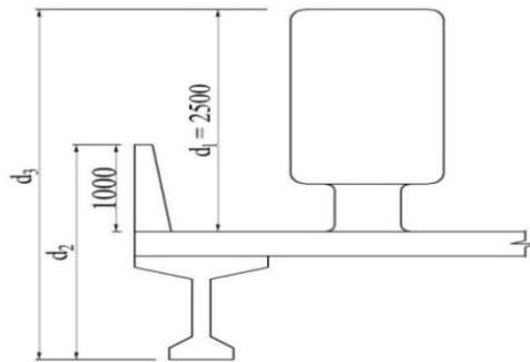
Fig 3.12 Wind Force Acting on the Bridge Deck (All dimensions in mm)
