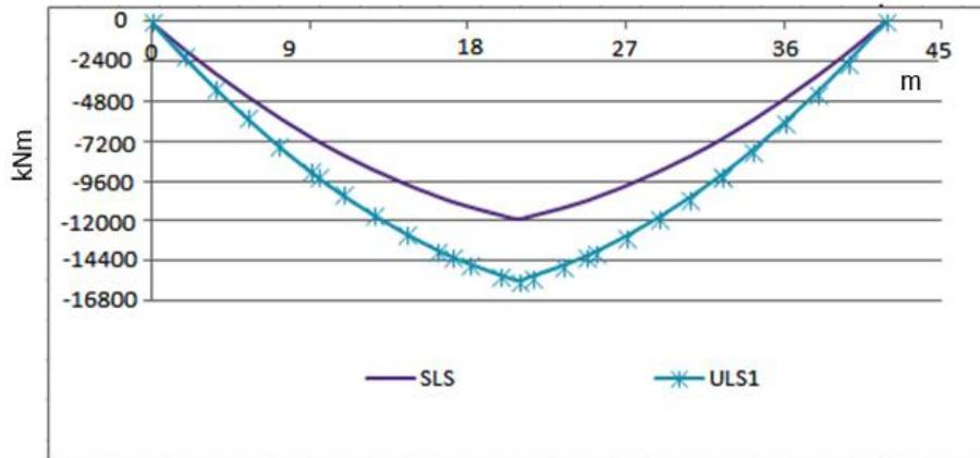
Fig 4.16 Moment Diagram for First Combination of Span 40m
