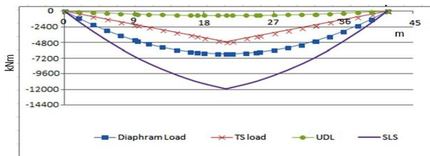
Fig 4.15 Moment Diagram of Span 40m
