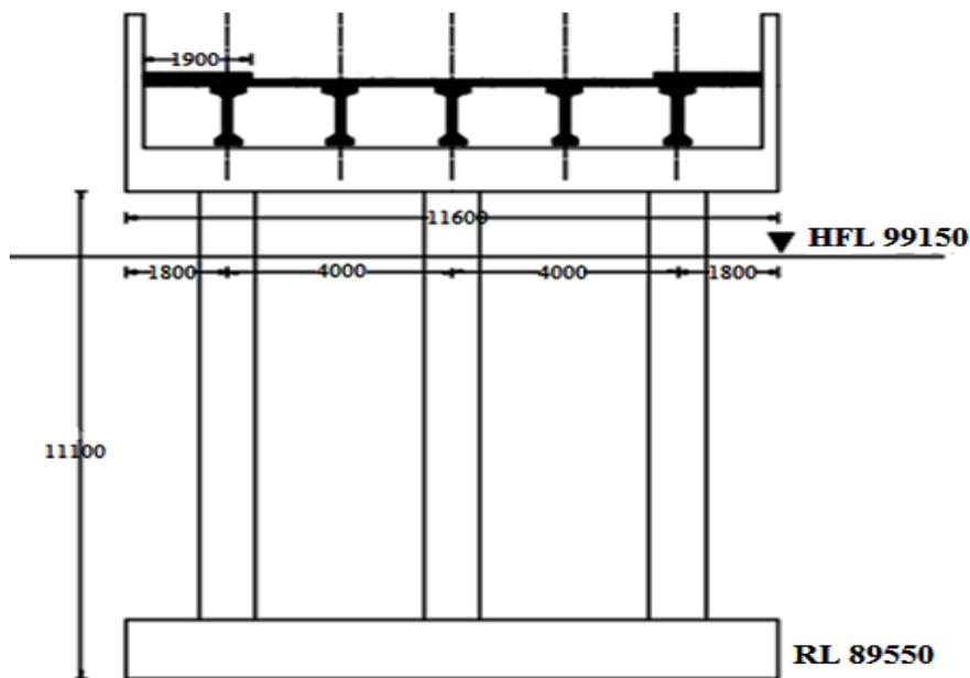
Fig 3.10 Typical Pier Cross Section (All dimensions in mm)
