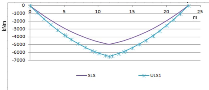
Fig 4.20 Moment at Middle of the Beam for First Combination Diagram of Span 23.2m
