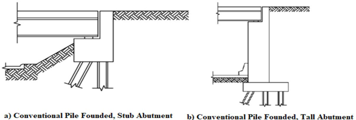
Fig 2.7 Conventional Abutments of Various Heights (FHWA, 2012)
