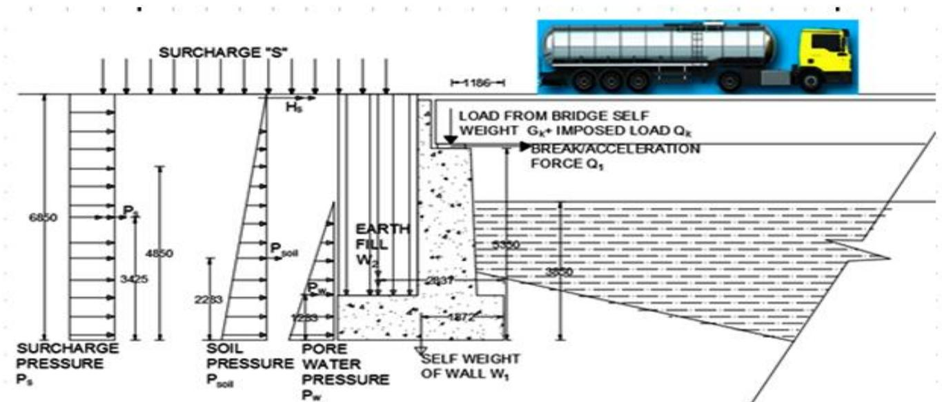
Fig 3.8 Active Forces on the Earth Retaining Wall side of the Abutment.
