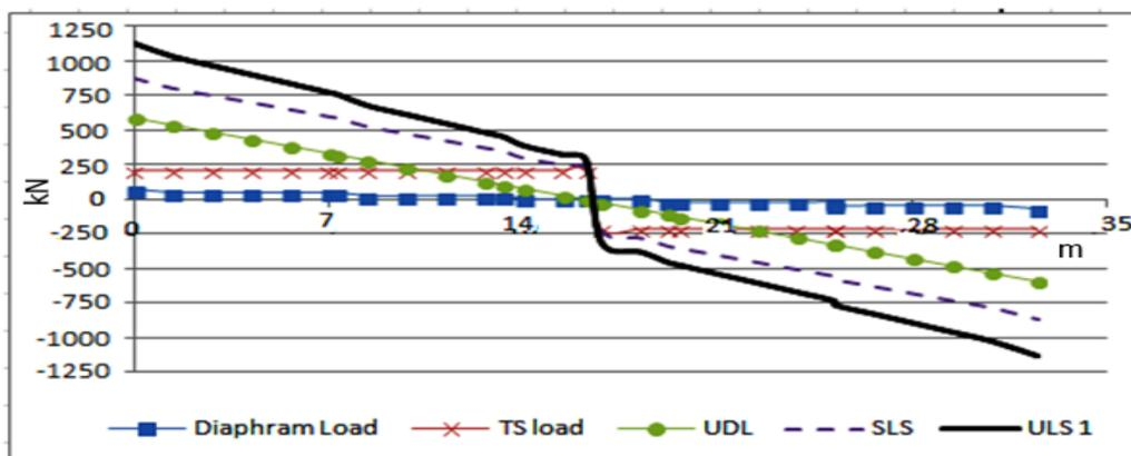
Fig 4.8 Shear Force Diagram of Span 30m
