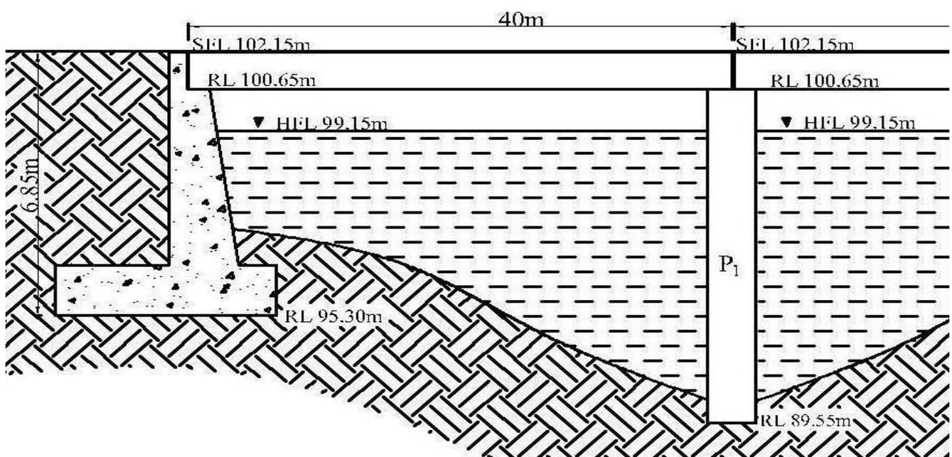
Fig 3.20 Pier position on Bridge Span of 40m
