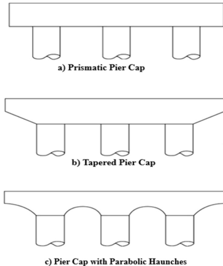
Fig 2.21 Different Types of Pier Caps for Multi-Column Piers (FHWA, 2012)
