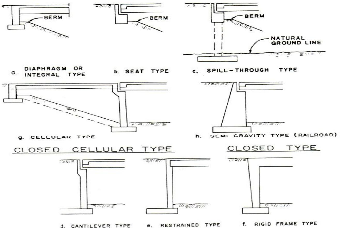
Fig 2.11 Typical Abutments (Anwar, 2015)
