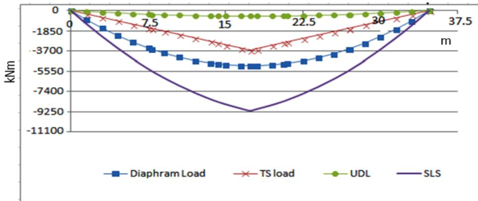
Fig 4.12 Moment diagram of Span 35m
