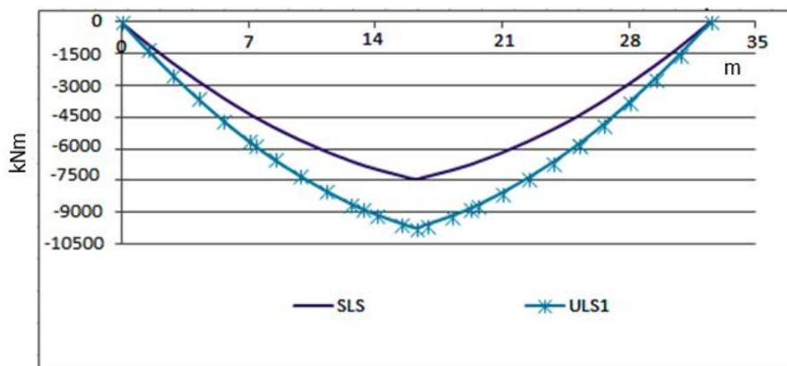
Fig 4.26 Moment at Middle of the Beam for First Combination Diagram of Span 30m
