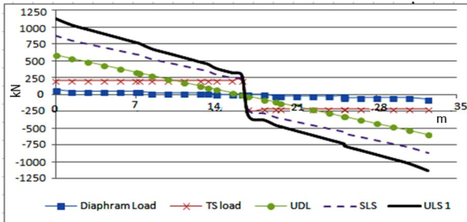
Fig 4.24 Shear Force Diagram of Span 30m
