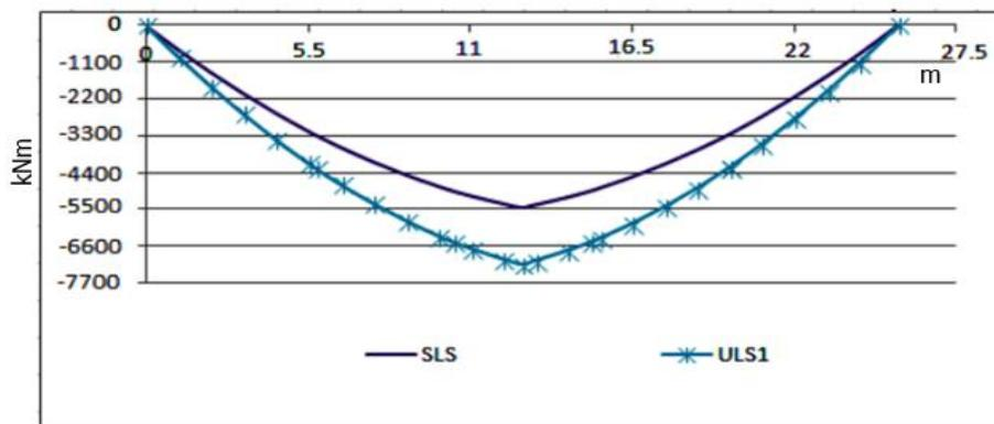
Fig 4.23 Moment at Middle of the Beam for First Combination Diagram of Span 25m
