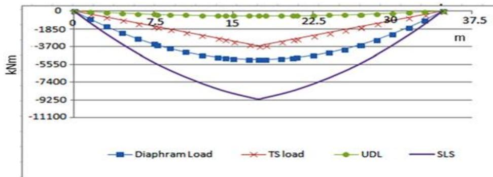
Fig 4.28 Moment Diagram of Span 35m
