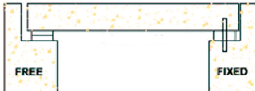
Fig 2.14 Free Abutment with Sliding Bearings (Childs, 2015)
