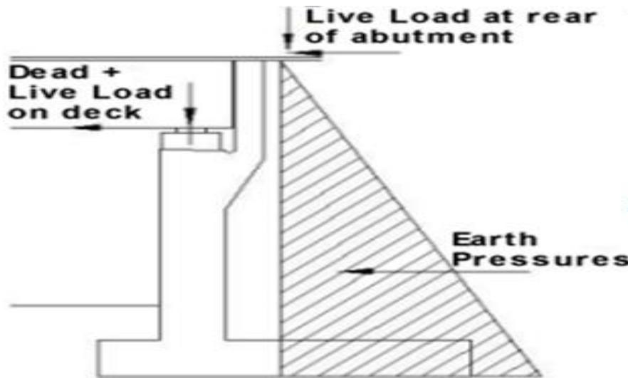
Fig 2.13 Abutment Loading (Childs, 2015)
