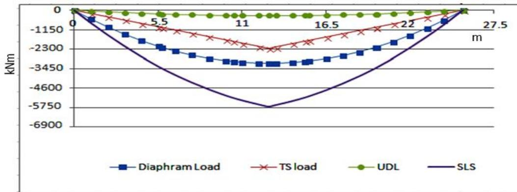
Fig 4.6 Moment Diagram of Span 25m
