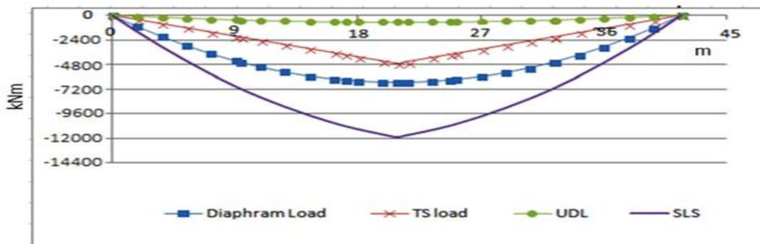
Fig 4.31 Moment Diagram of Span 40m
