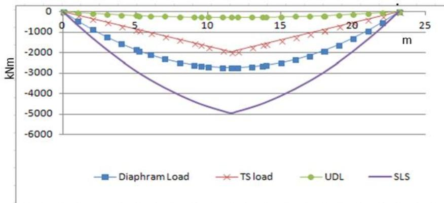
Fig 4.19 Moment Diagram of Span 23.2m
