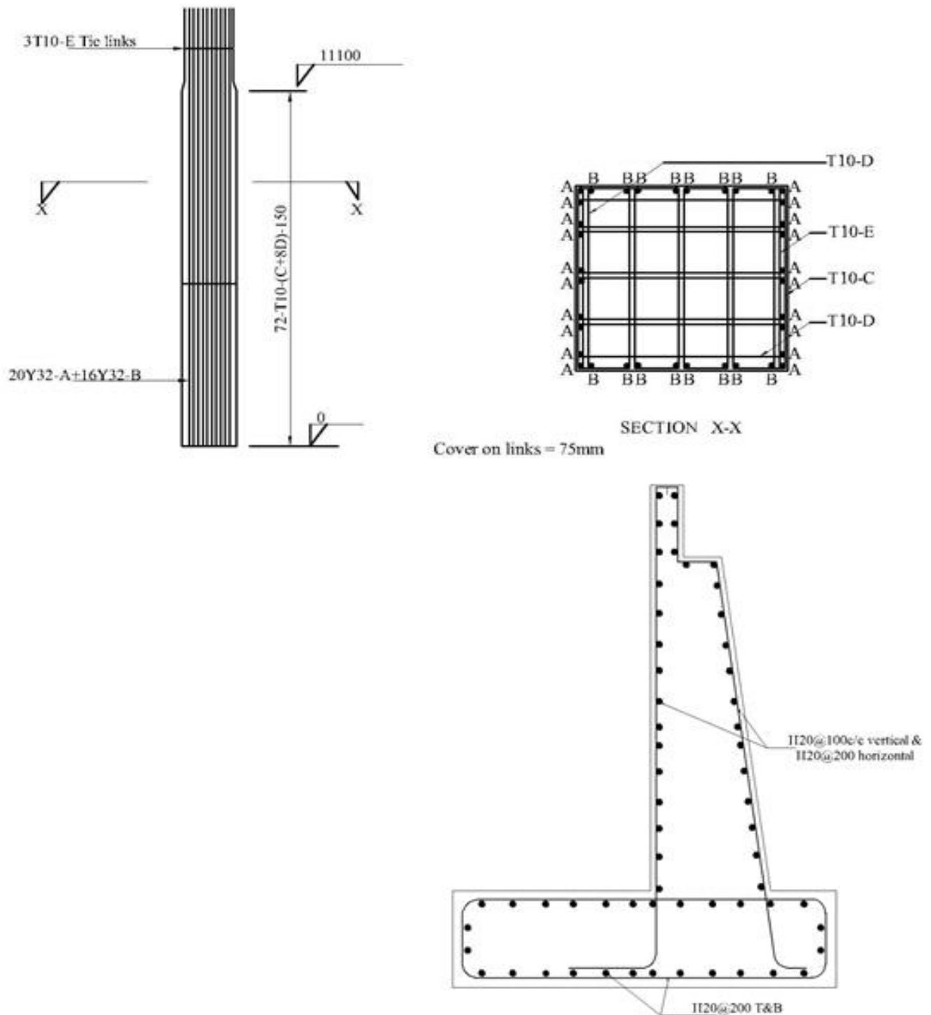
Fig 4.17 Detailing of the Abutment and Pier
