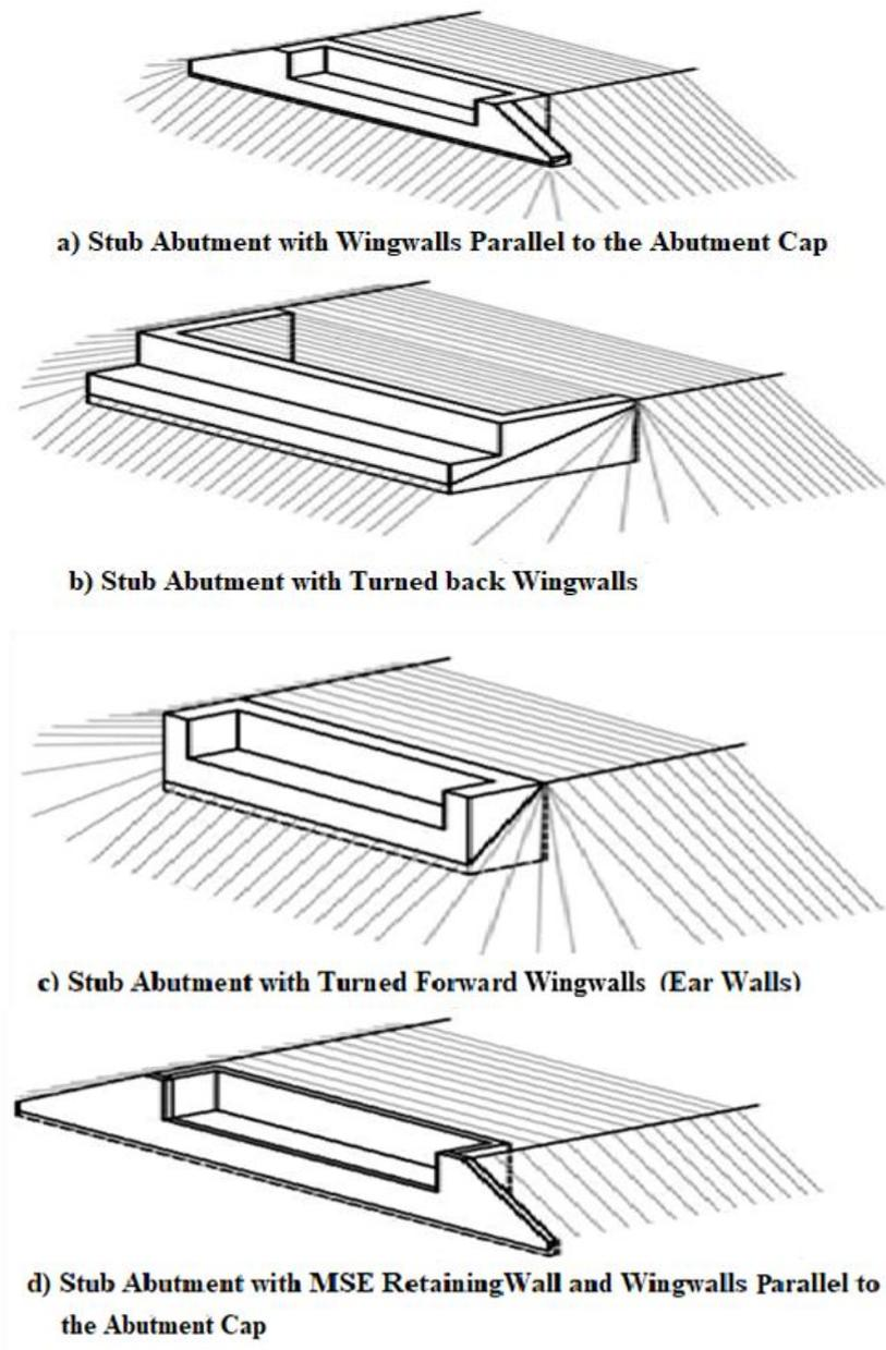
Fig 2.8 Abutment Wingwall Configurations (FHWA, 2012)
