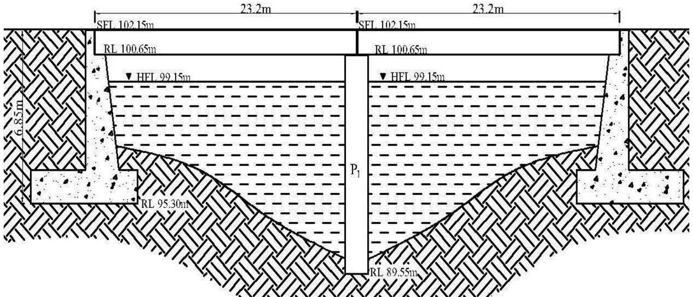
Fig 3.1 Typical Bridge Section
