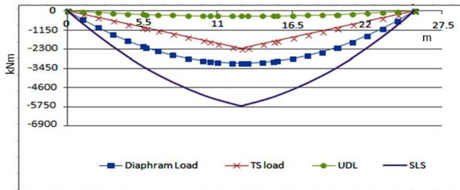
Fig 4.22 Moment Diagram of Span 25m
