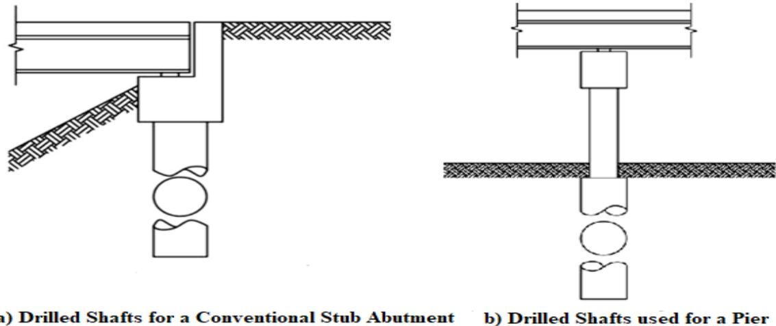
Fig 2.6 Drilled Shaft Applications (FHWA, 2012)
