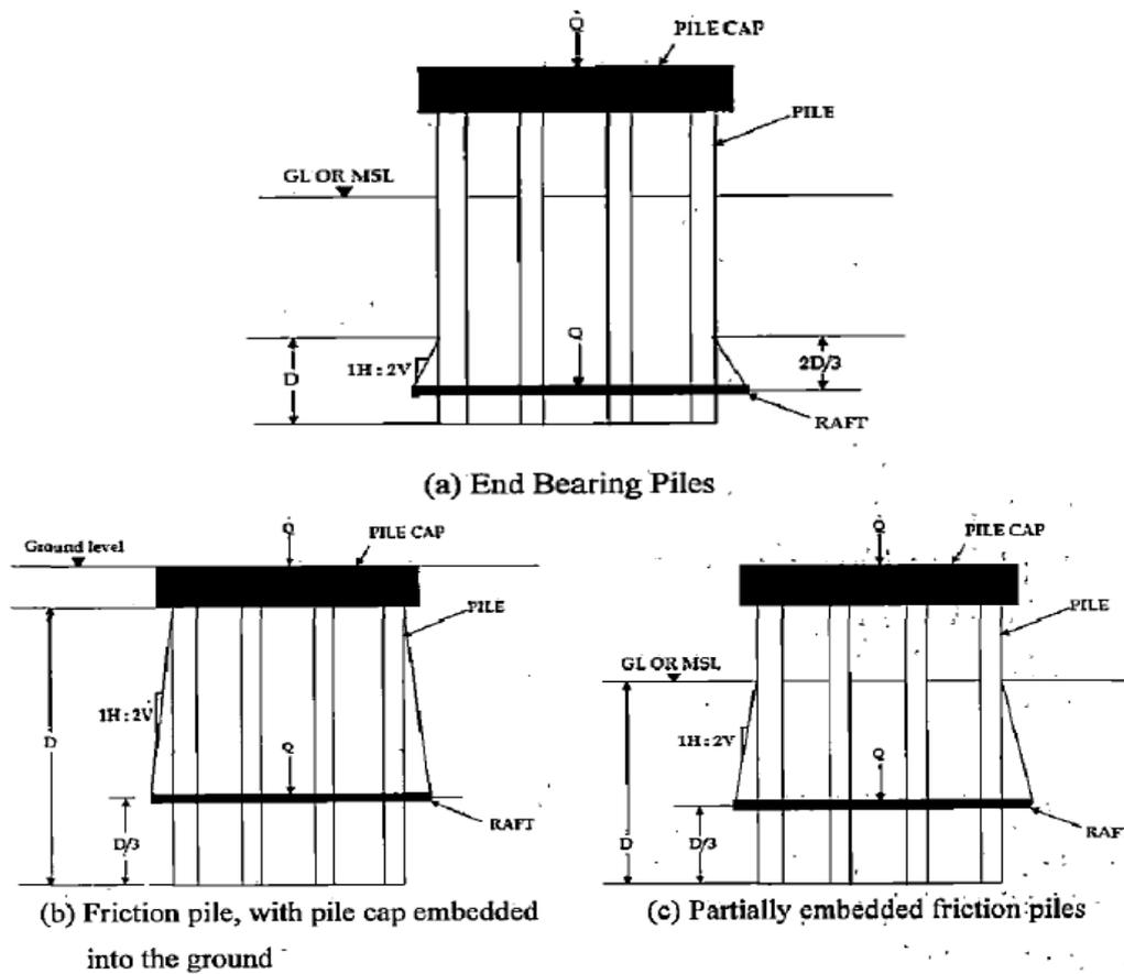
Fig 2.4 Computation of Settlement for end bearing Piles & Friction Piles (Terzaghi and Peck (1967))
