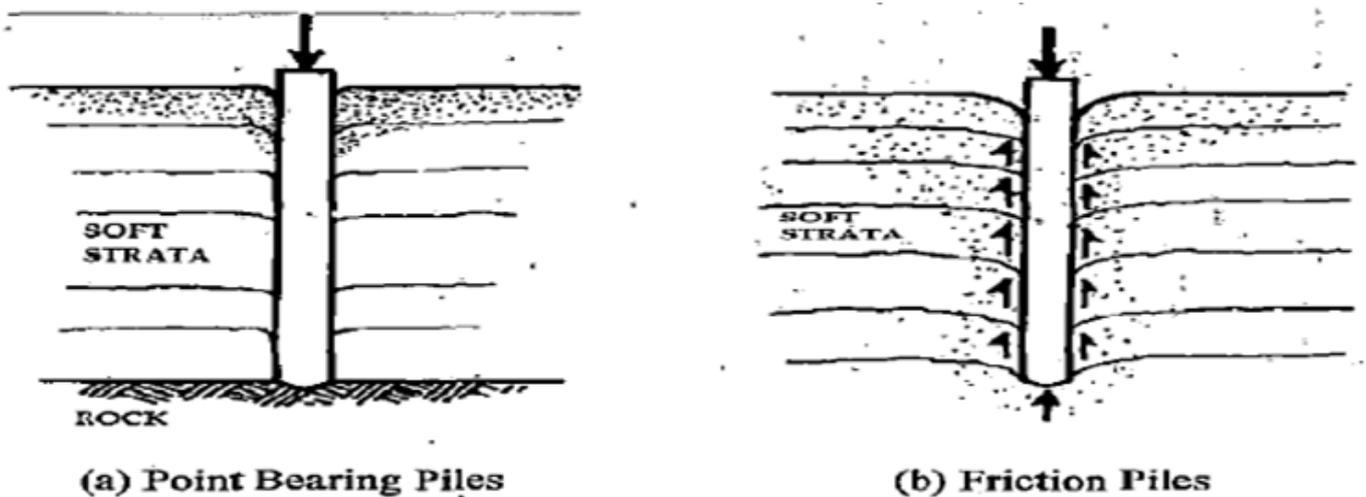
Fig 2.3 Pile Classifications on the Basis of Load Transfer Mechanism (Patel, 2008).
