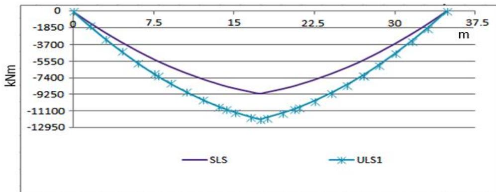
Fig 4.13 Moment Diagram for First Combination of Span 35m
