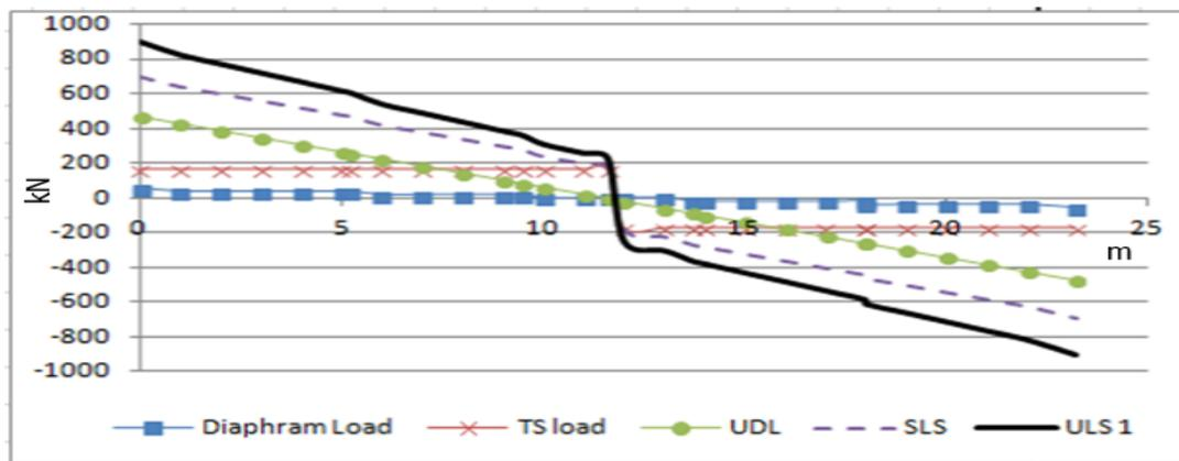
Fig 4.1 Shear Force Diagram of Span 23.2m
