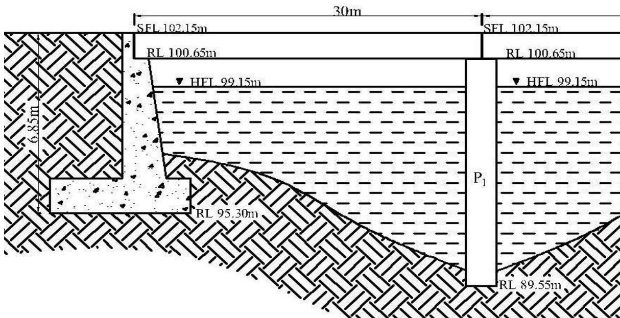
Fig 3.16 Pier Position on Bridge Span of 30m
