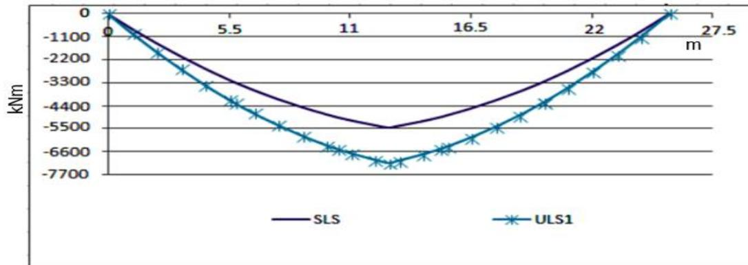
Fig 4.7 Moment diagram for first combination of Span 25m
