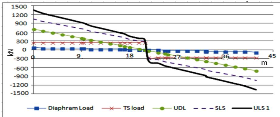
Fig 4.30 Shear Force Diagram of Span 40m
