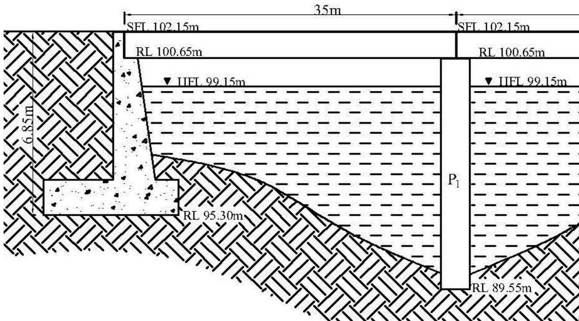
Fig 3.18 Pier Position on Bridge Span of 35m
