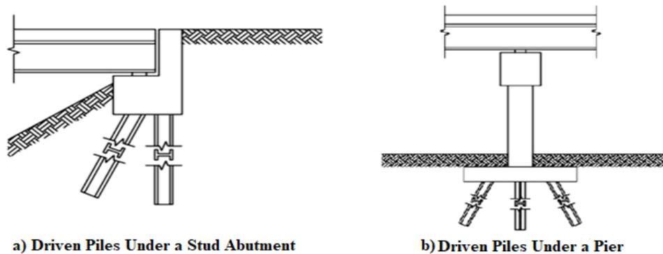
Fig 2.2 Driven Pile Applications (FHWA, 2012)
