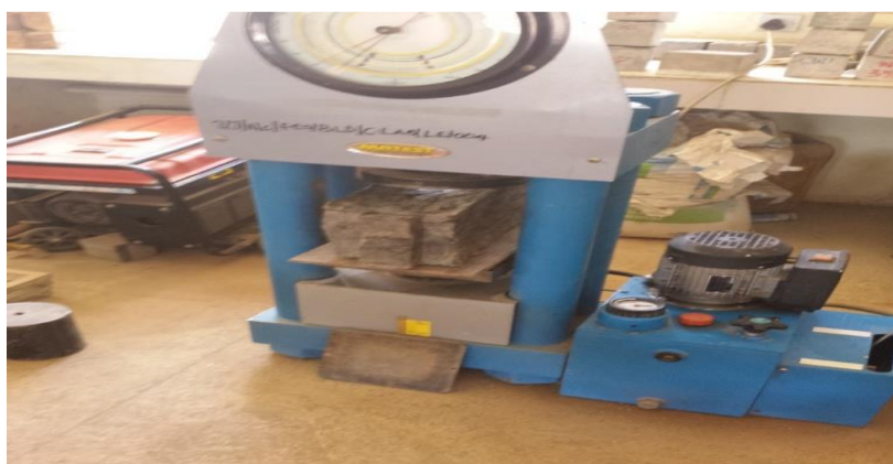
Fig. 4: Crushing of PSWB for Compressive Strength
