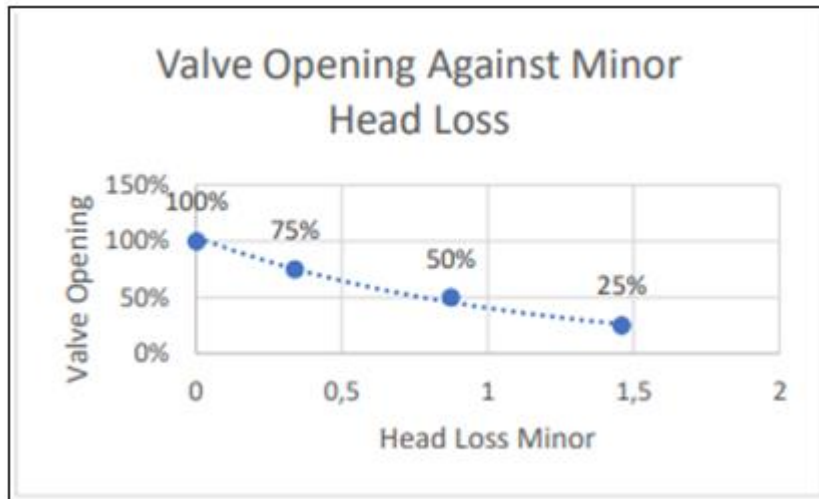
Fig 4 Valve Opening Against Minor Head Loss
