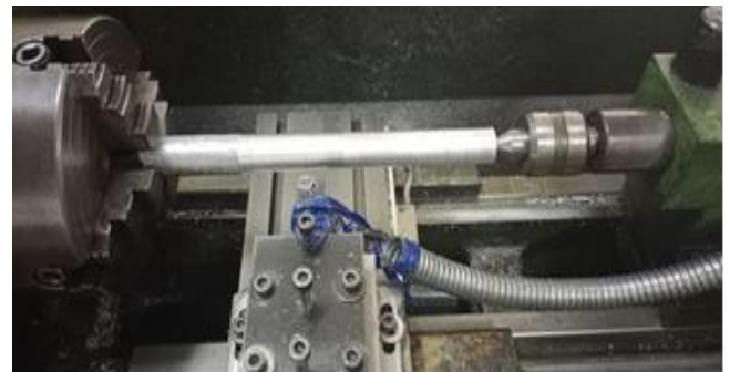
Fig 1 Measurement of Depth of Cut During Turning
