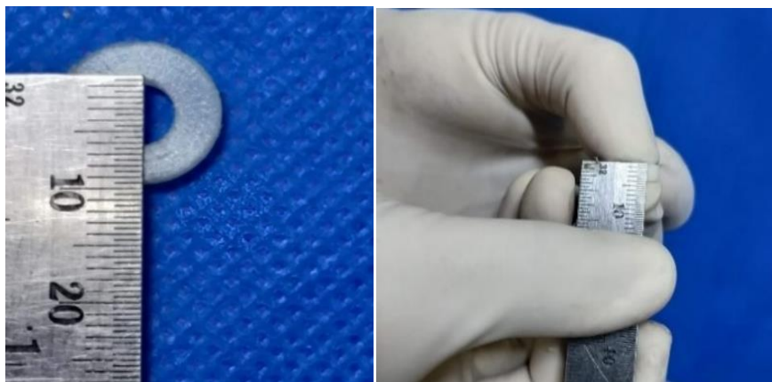
Fig. 2: Molds measuring 6.0 \pm 0.1 mm in diameter and 3.0 \pm 1.0 mm in thickness (ISO Standard 9917)
