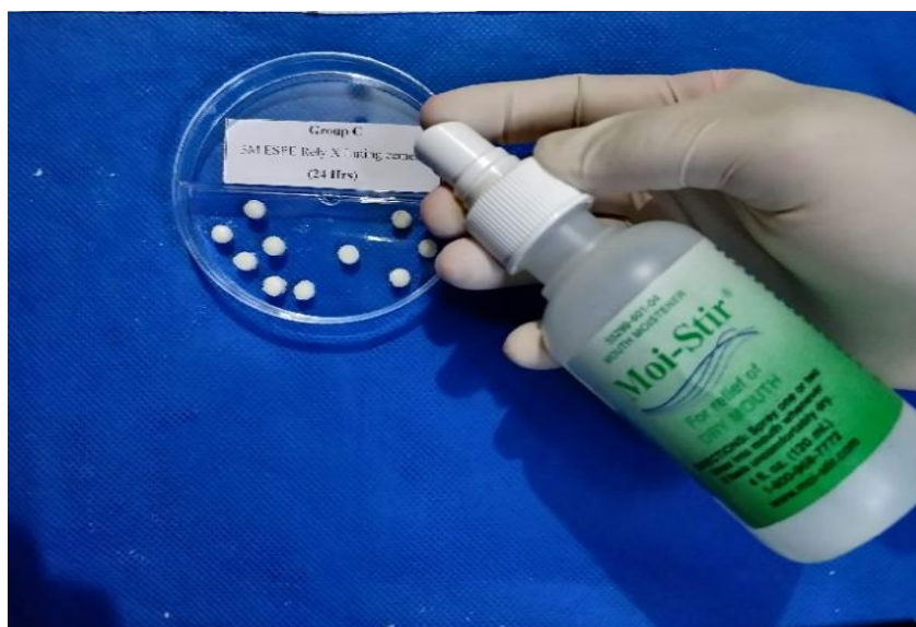
Fig. 8: The samples are placed in Artificial saliva
