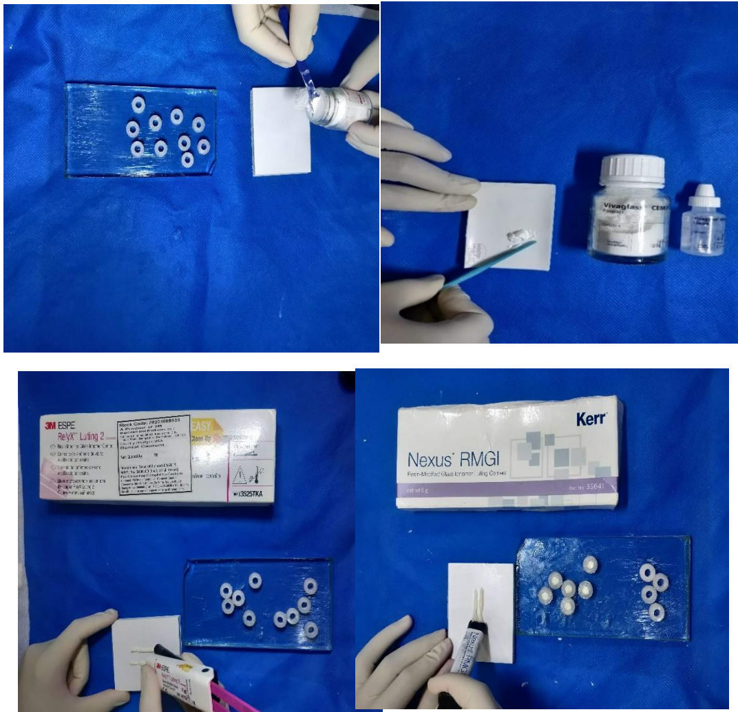
Fig. 5: Cements are mixed according to manufacturer’s instructions
