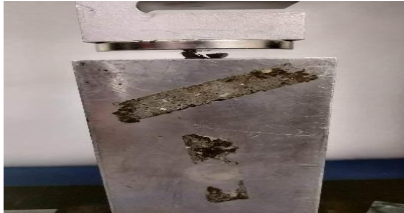
Fig 14: Specimen after fracture under diametral tensile load
