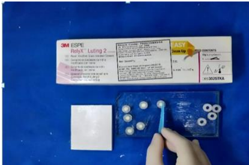
Fig 6: The mixed cements are immediately poured into the molds
