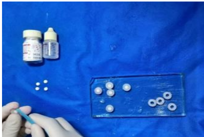
Fig. 7: Specimens are carefully removed from the molds
