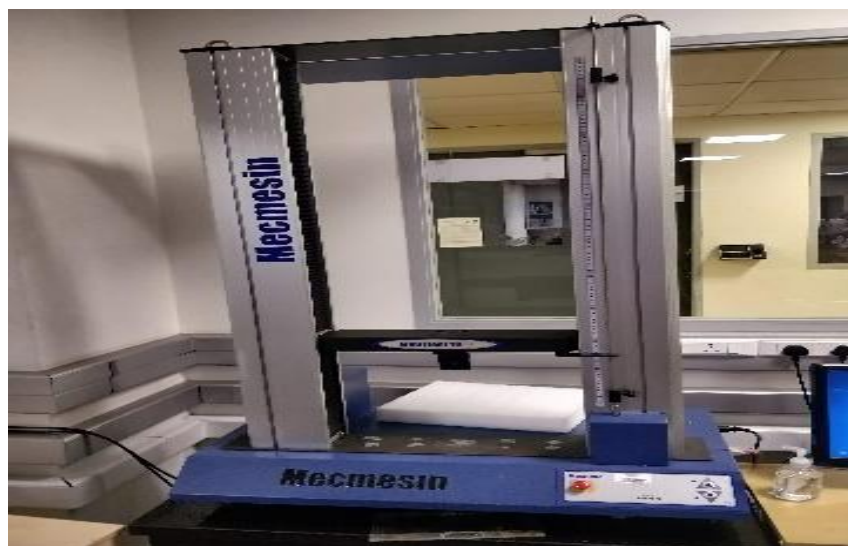
Fig. 12: Universal Testing Machine (UTM) for Diametral Tensile strength testing (Mecmesin Multitest 10-i)
