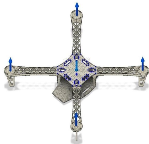
Fig. 4: Meshed frame with load
