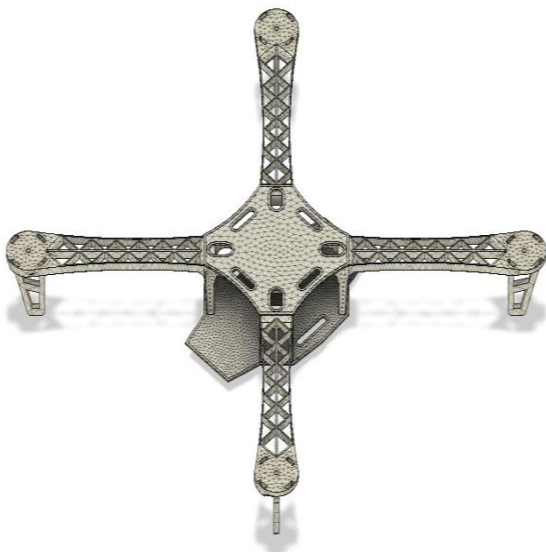
Fig. 3: Mesh results for frame structure
