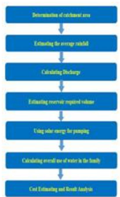
Fig 6 Methodology of the Rainwater Harvesting
